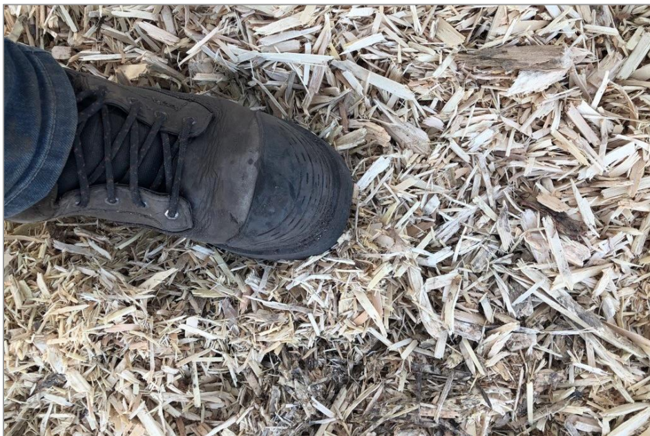
Photo 6 Material described as 2-inch hog fuel. (Photo Courtesy of Ledcor)
