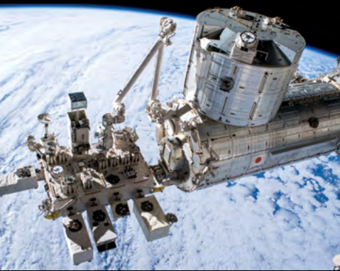
Space station's view of Earth helps farmers water crops, supports disaster response, monitors climate, and more. Seen here is the suite of Earth-observing payloads attached to the Japanese Experiment Module.
