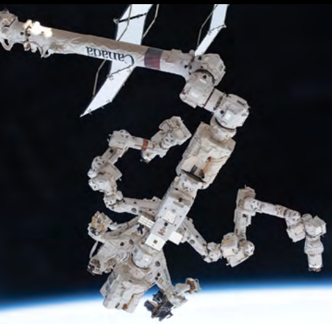
The Canadian Space Agency's Special Purpose Dexterous Manipulator, also known as Dextre, is pictured attached to the International Space Station's Canadarm2 robotic arm. Dextre is the orbiting lab's fine-tuned robotic hand, designed for precise handling abilities and routine maintenance tasks such as replacing batteries and cameras in the harsh environment of space.
