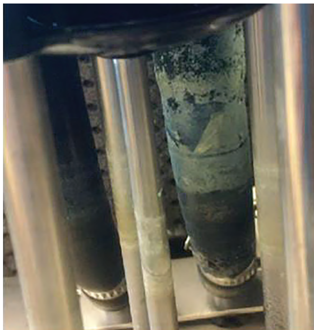
Figure 2. Biofilm visualized on surfaces submerged in an internal water reservoir of a heater-cooler device during investigation of invasive extrapulmonary nontuberculous mycobacteria infections among patients who underwent cardiothoracic surgery, York, Pennsylvania, USA, 2015.
