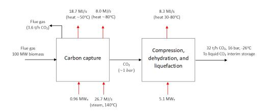
Figure 10. Illustration of energy balance for a  $CO_2$  capture and liquefaction plant treating all flue gas from a 100 MWth biomass boiler that is equipped with flue gas condensation. 90% of the  $CO_2$  in the flue gas is captured corresponding to 32 t  $CO_2$  output per hour. Black arrows: Mass streams. Red arrows: Energy streams.
