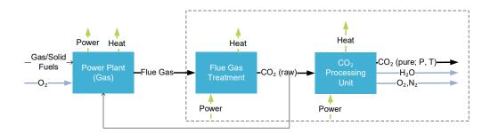
Figure 5: Oxy-fuel combustion
