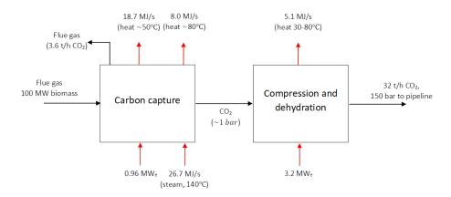
Figure 9. Illustration of energy balance for a  $CO_2$  capture and compression plant treating all flue gas from a 100 MW<sub>th</sub> biomass boiler that is equipped with flue gas condensation. 90% of the  $CO_2$  in the flue gas is captured corresponding to 32 t  $CO_2$  output per hour. Black arrows: Mass streams. Red arrows: Energy streams.
