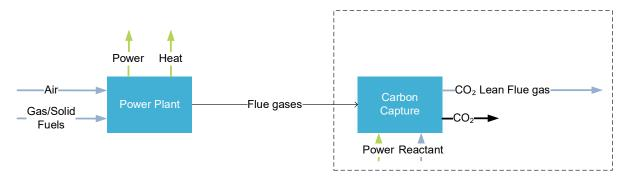
Figure 3: Post combustion
