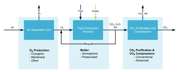
Figure 17 Schematic illustration of oxy-fuel combustion.[1]
