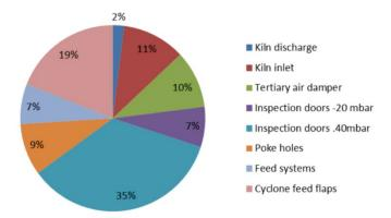
Figure 21 Overview of air-leakages in the preheater and kiln departments at a typical Portland cement plant.[5]
