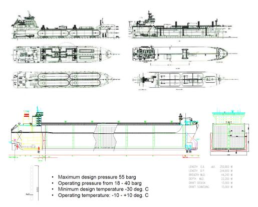
Figure 66. Top) Sketch of refrigerated CO<sub>2</sub> ship designs for Gassco Concept study [12]. Bottom) sketch of Knutsen Shipping's design of a pressurised CO<sub>2</sub> carrier (PCO<sub>2</sub>) [13].
