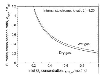
Figure 29 Potential to reduce boiler size by increasing O<sub>2</sub> concentration.[14]
