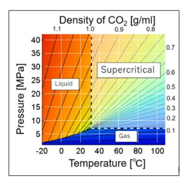
Figure 64. CO<sub>2</sub> density at varying pressure and temperature Image source: ITEC Co., Ltd. Osaka, Japan.
