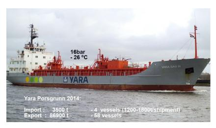
Figure 49. M/T Yara Gas III liquid CO<sub>2</sub> carrier. [7]
