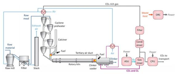
Figure 19: Cement kiln system converted to oxy-fuel firing. The reddish coloured blocks are new process units.[3, 4]
