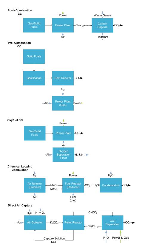
Figure 2: Simplified block flow diagrams of the various CC systems described herein.[1]
