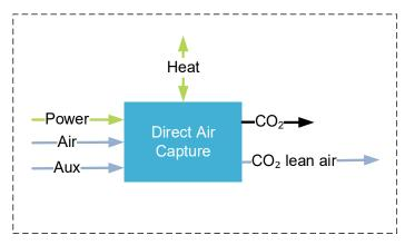
Figure 6. Illustration of Direct Air Capture (DAC).
