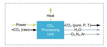
Figure 7. Illustration of CO<sub>2</sub> processing (conditioning) unit.
