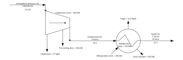
Figure 58: Example of the energy balance for a CO<sub>2</sub> compression and liquefaction plant.
