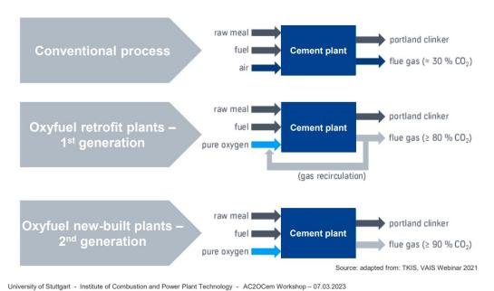
Figure 18 Schematic representation of conventional, 1 and 2. G oxyfuel cement plants.[2]
