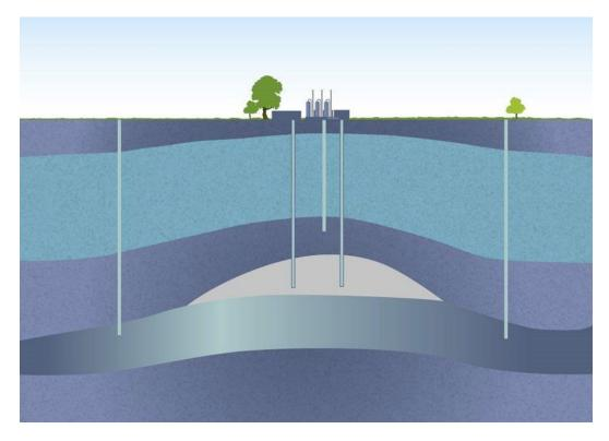
Figure 0-8: Schematic illustration of a storage site with central injection wells and observation wells placed to monitor the flanks and the spill-point of the structure [9]
