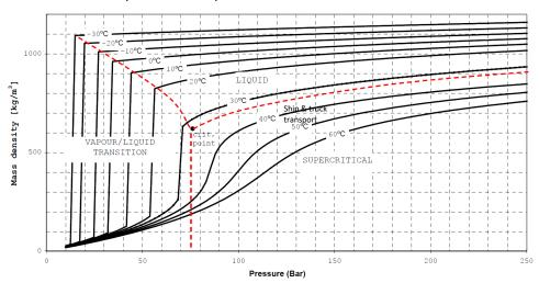
Figure 46. Mass density of pure CO<sub>2</sub> as function of pressure based on Peng-Robinson EQS. Source: DNV-GL RP-J202.
