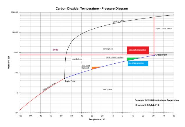
Figure 45. CO<sub>2</sub> phase diagram with the options for liquid-, gas- and dense phase transportation.
