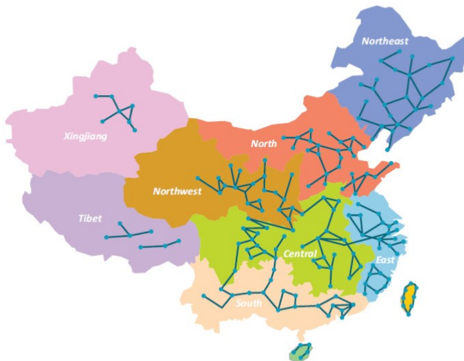
Figure 1: Regional power grid clusters in China . Source: Market potential and technology transfer, NDRC Energy Research Institute, November 2009
