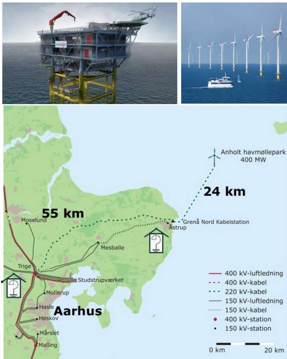
Figure 56: Connection of Anholt 400 MW offshore wind farm
