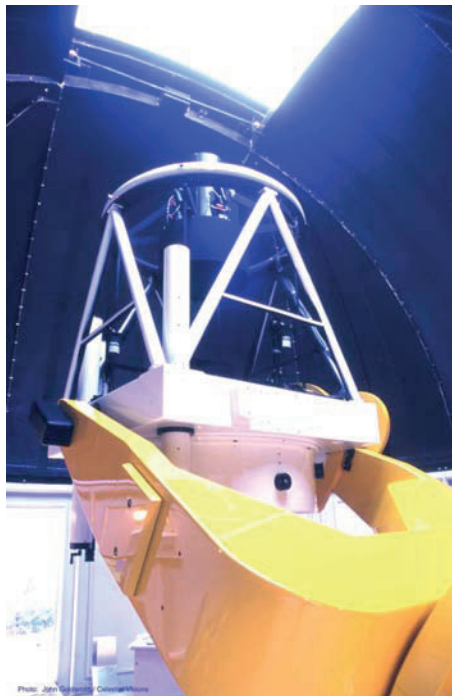
Fig. 1 – The 1-m f/4 Cassegrain Zadko Telescope is fully robotic and employs the same control software as the TAROT telescopes (located in France and Chile). An automated image processing pipeline produces calibrated FITS images to external users via a web-based interface.
