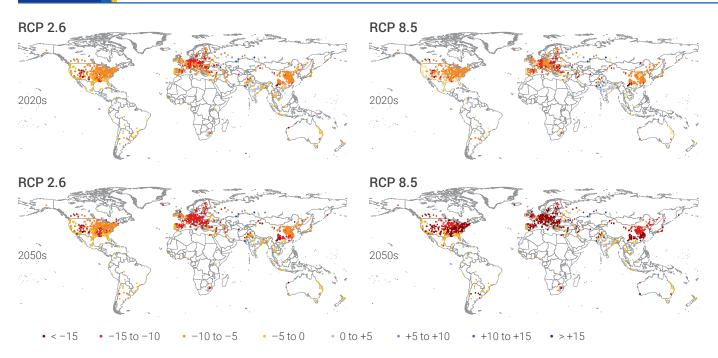
*Notes*: Relative changes in annual mean usable capacity of thermoelectric power plants for RCP 2.6 and RCP 8.5 for 2010–39 (2020s) and 2040–69 (2050s) relative to the control period 1971–2000.
