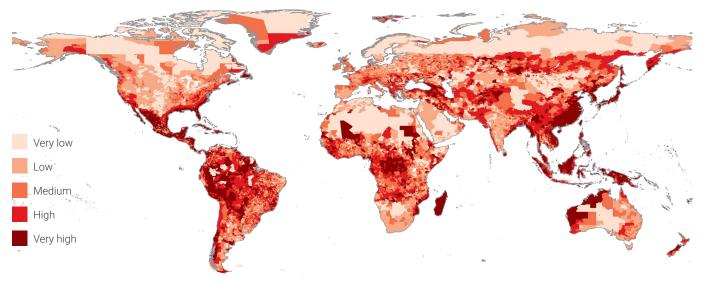
*Notes*: The classification is based on 20th percentiles of road and rail assets that are exposed to flood hazards. *Source*: Koks et al., 2019.<sup>83</sup>
