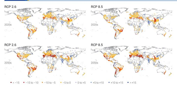
Notes: Relative changes in annual mean usable capacity of hydropower plants for RCP 2.6 and RCP 8.5 for 2010–39 (2020s) and 2040–69 (2050s) relative to the control period 1971–2000.
