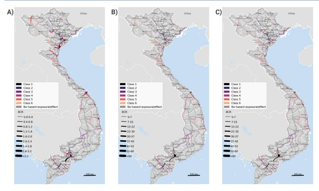
*Notes*: Comparisons of BCRs of adaptation options for national-scale road network links in Vietnam subjected to A) current 2016 levels of extreme river flooding, and future 2030 levels of extreme river flooding under B) RCP 4.5 and C) RCP 8.5.
