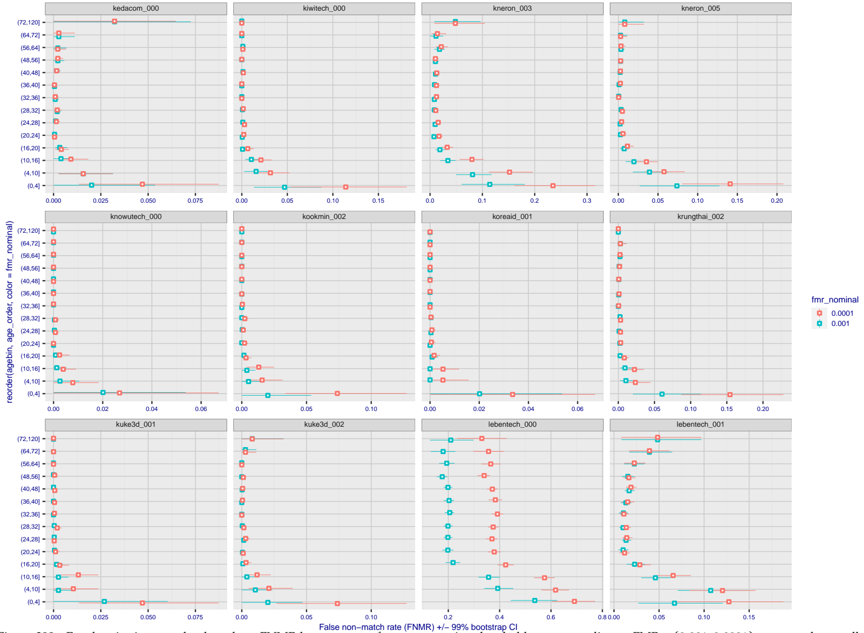
Figure 390: For the visa images, the dots show FNMR by age group for two operating thresholds corresponding to FMR = \{0.001, 0.0001\} computed over all on the order of 10^{10} impostor scores. The FMR in each bin will vary also - see subsequent impostor heatmaps in sec. 3.6.2. Given a pair of face images taken at different times, we assign the comparison to the bin that is the arithmetic average of the subject's ages. This plot shows only the effect of age, not ageing. The number of comparisons in each bin is generally in the thousands, however the first and last bins are computed over 149 and 124 respectively. The error rates in some (adult) cases are zero, and in others the DET is flat so the error rates at the two thresholds are identical. The lines span 1% and 99% of bootstrap replicated FNMR estimates.
