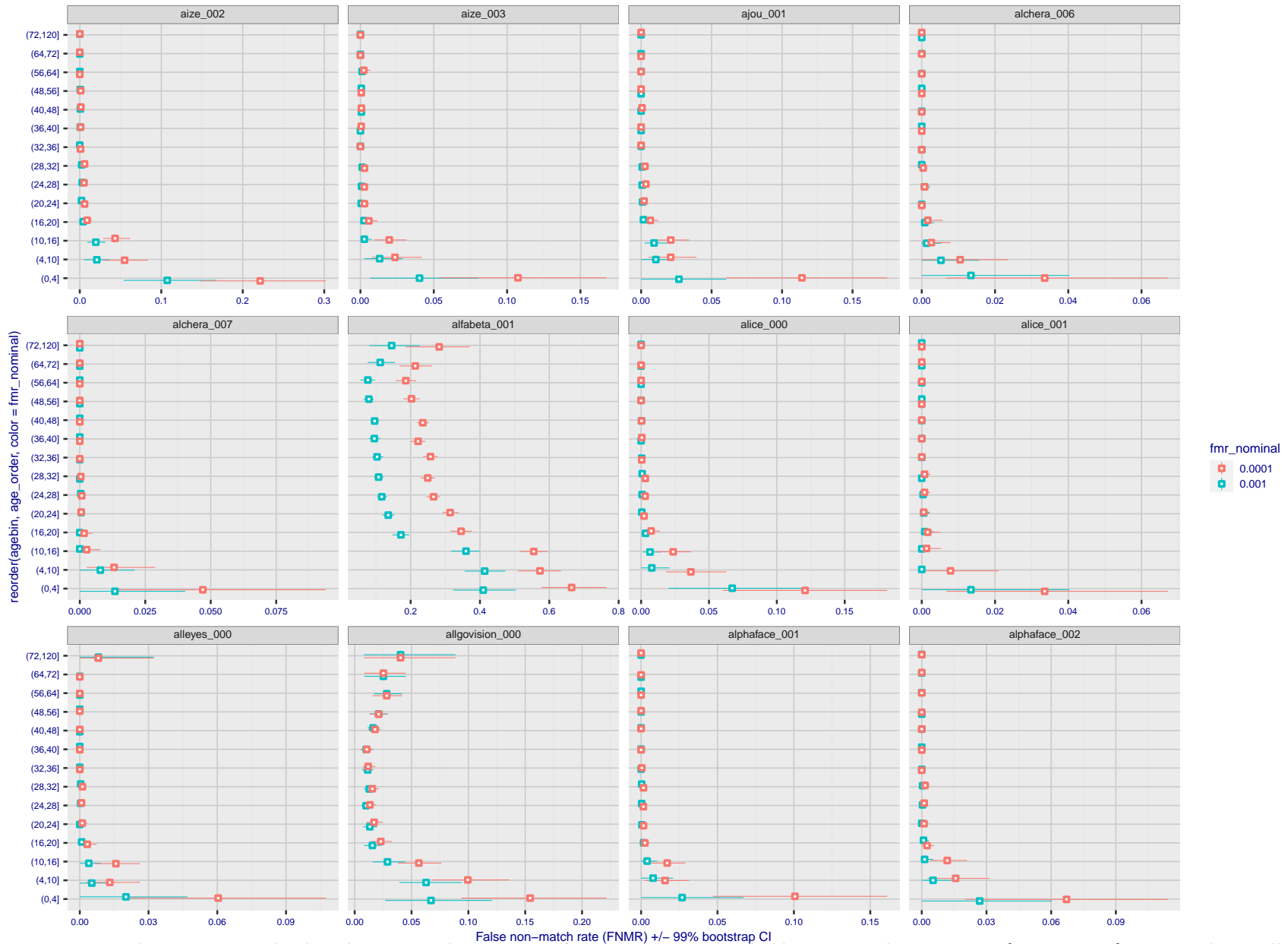
Figure 370: For the visa images, the dots show FNMR by age group for two operating thresholds corresponding to FMR = \{0.001, 0.0001\} computed over all on the order of 10^{10} impostor scores. The FMR in each bin will vary also - see subsequent impostor heatmaps in sec. 3.6.2. Given a pair of face images taken at different times, we assign the comparison to the bin that is the arithmetic average of the subject's ages. This plot shows only the effect of age, not ageing. The number of comparisons in each bin is generally in the thousands, however the first and last bins are computed over 149 and 124 respectively. The error rates in some (adult) cases are zero, and in others the DET is flat so the error rates at the two thresholds are identical. The lines span 1% and 99% of bootstrap replicated FNMR estimates.
