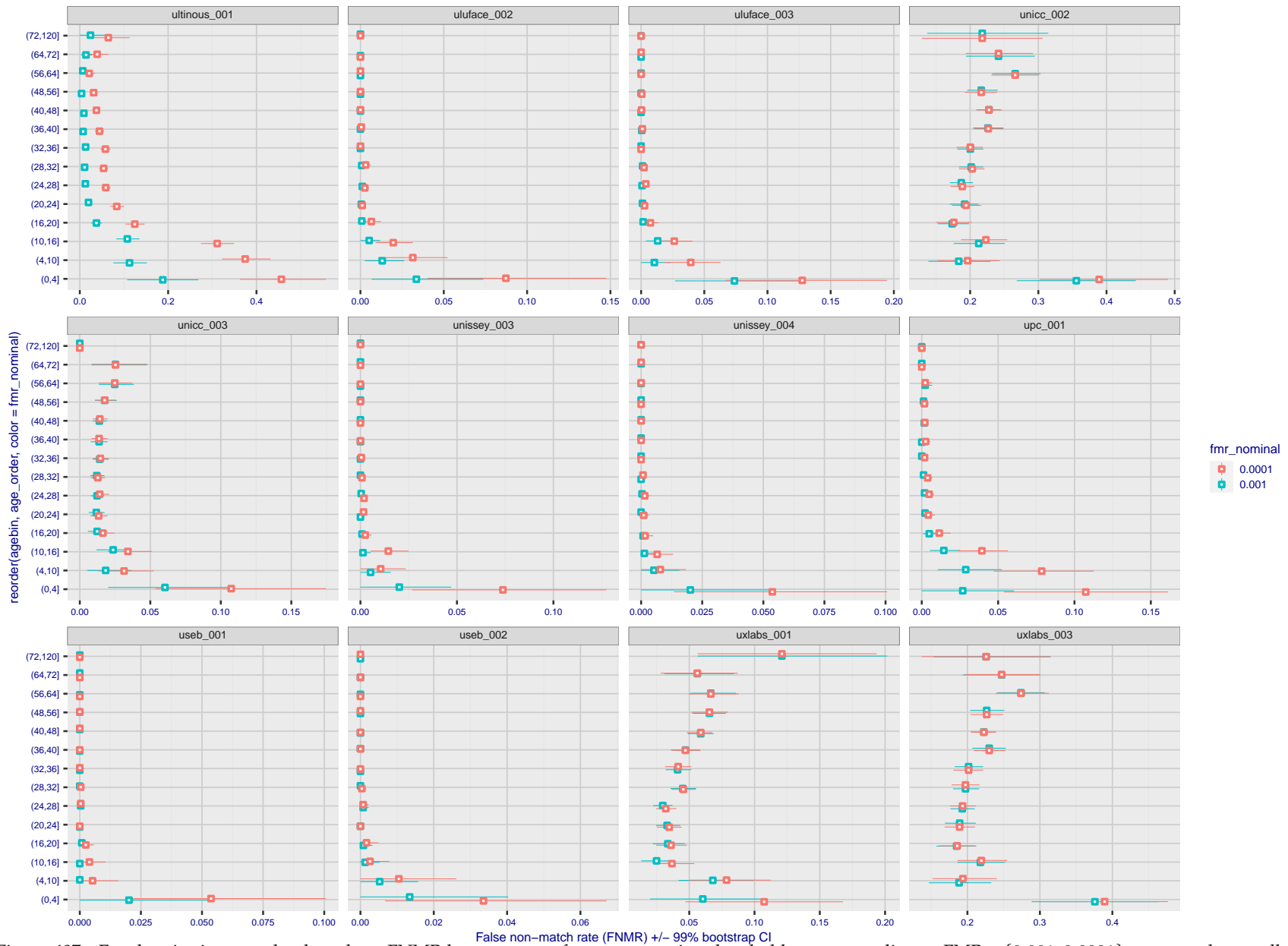
Figure 407: For the visa images, the dots show FNMR by age group for two operating thresholds corresponding to FMR = \{0.001, 0.0001\} computed over all on the order of 10^{10} impostor scores. The FMR in each bin will vary also - see subsequent impostor heatmaps in sec. 3.6.2. Given a pair of face images taken at different times, we assign the comparison to the bin that is the arithmetic average of the subject's ages. This plot shows only the effect of age, not ageing. The number of comparisons in each bin is generally in the thousands, however the first and last bins are computed over 149 and 124 respectively. The error rates in some (adult) cases are zero, and in others the DET is flat so the error rates at the two thresholds are identical. The lines span 1% and 99% of bootstrap replicated FNMR estimates.
