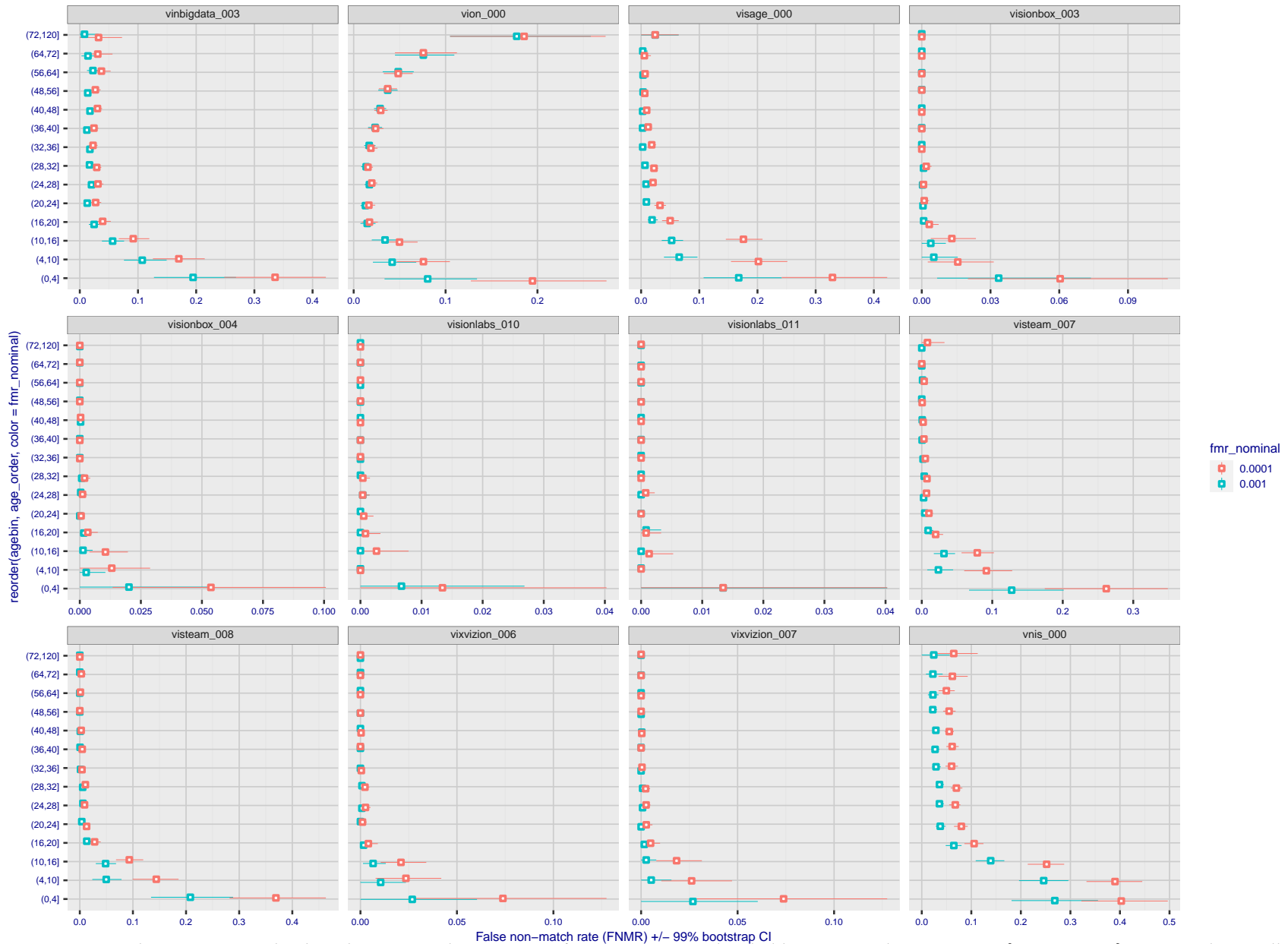
Figure 410: For the visa images, the dots show FNMR by age group for two operating thresholds corresponding to FMR = \{0.001, 0.0001\} computed over all on the order of 10^{10} impostor scores. The FMR in each bin will vary also - see subsequent impostor heatmaps in sec. 3.6.2. Given a pair of face images taken at different times, we assign the comparison to the bin that is the arithmetic average of the subject's ages. This plot shows only the effect of age, not ageing. The number of comparisons in each bin is generally in the thousands, however the first and last bins are computed over 149 and 124 respectively. The error rates in some (adult) cases are zero, and in others the DET is flat so the error rates at the two thresholds are identical. The lines span 1% and 99% of bootstrap replicated FNMR estimates.
