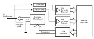
Figure 2: the oscillator experimental setup
