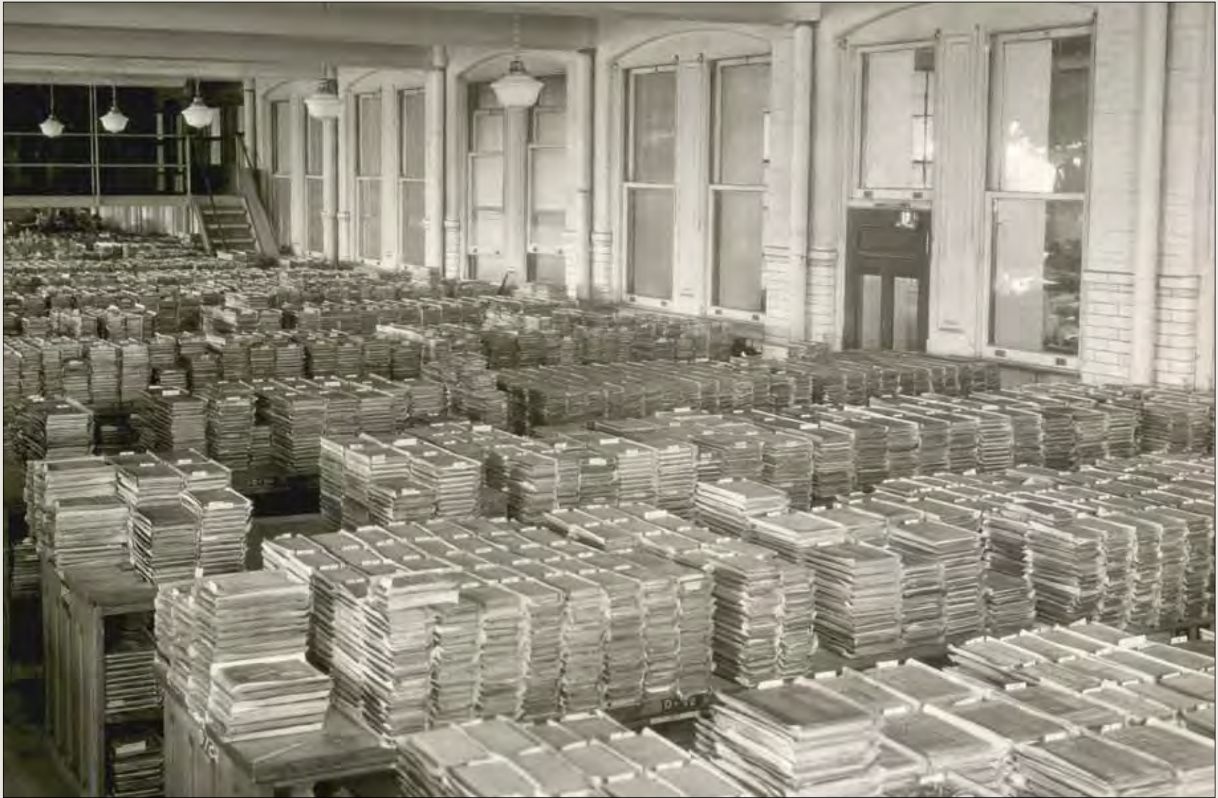
Once plates were struck, the imposed pages were often “pied” — broken up for the typemetal to be reused. If the order was for a particularly large run, or additional quantities were likely, the type was left standing and stored in anticipation of making further plates and pressruns. Photo circa 1930.
