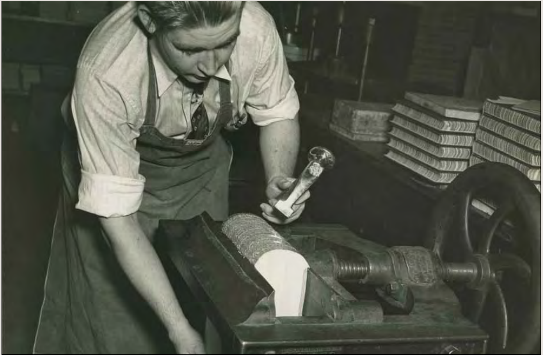
An apprentice works at rounding and backing a sewn and glued bookblock, prior to its being secured in hardback covers.
