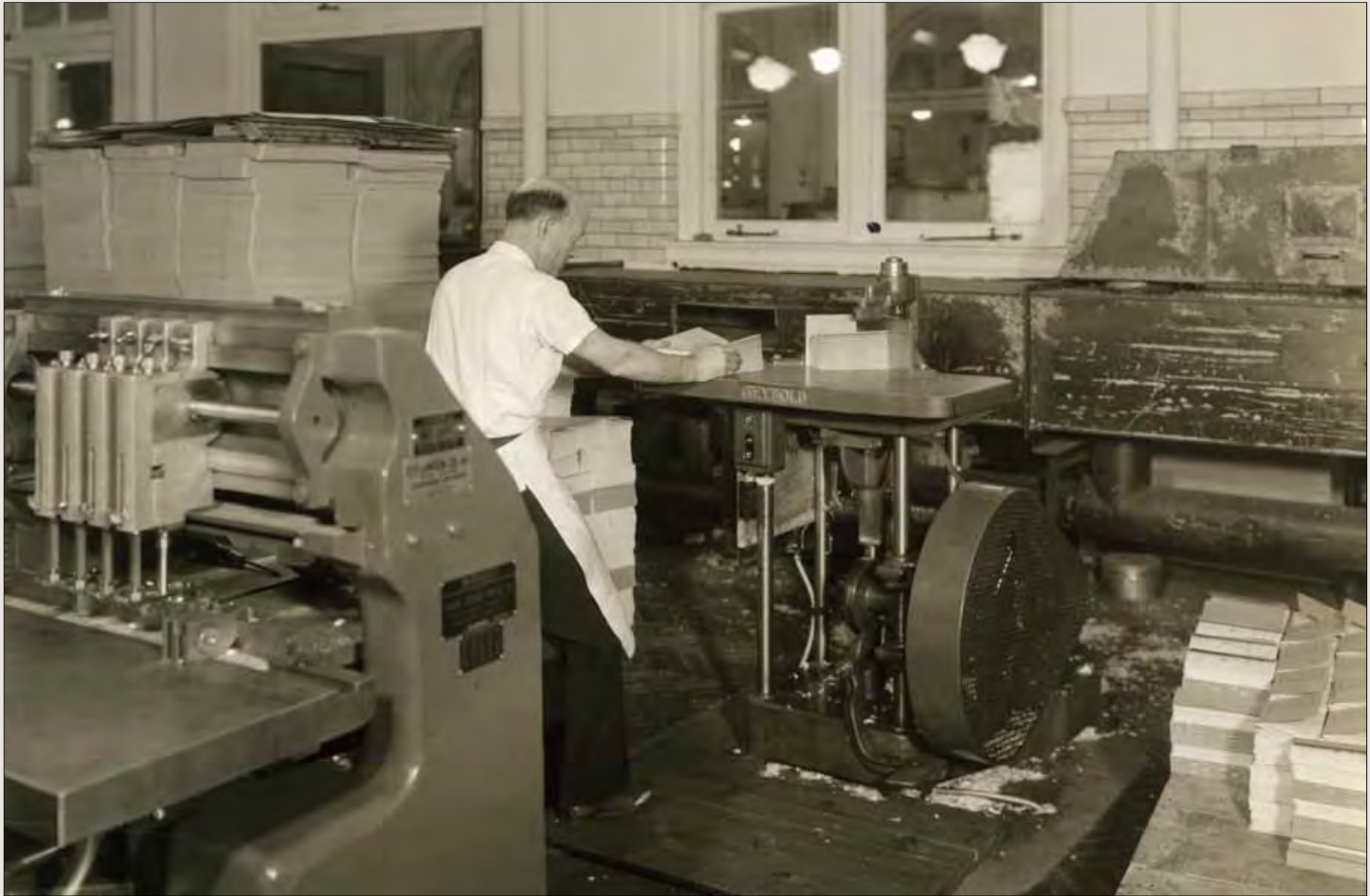
A bookbinder operates a machine for cutting rounded corners in this photo from the 1940s. The machine at left is a drill for pages to be inserted in ring binders.
