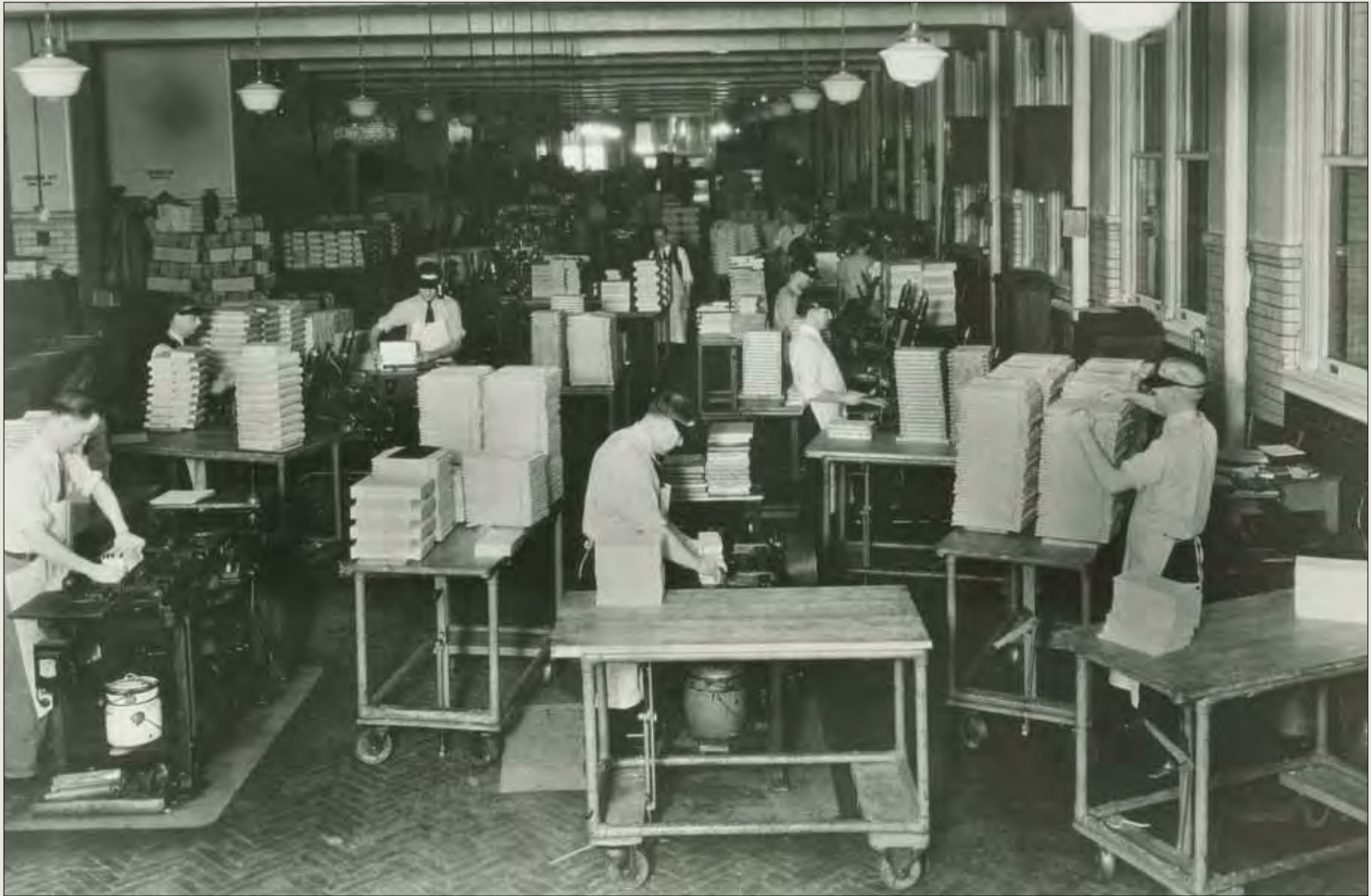
Bookbinders rounding and backing sewn bookblocks during the 1930s with machines that shaped the spine and applied adhesive for backing material.
