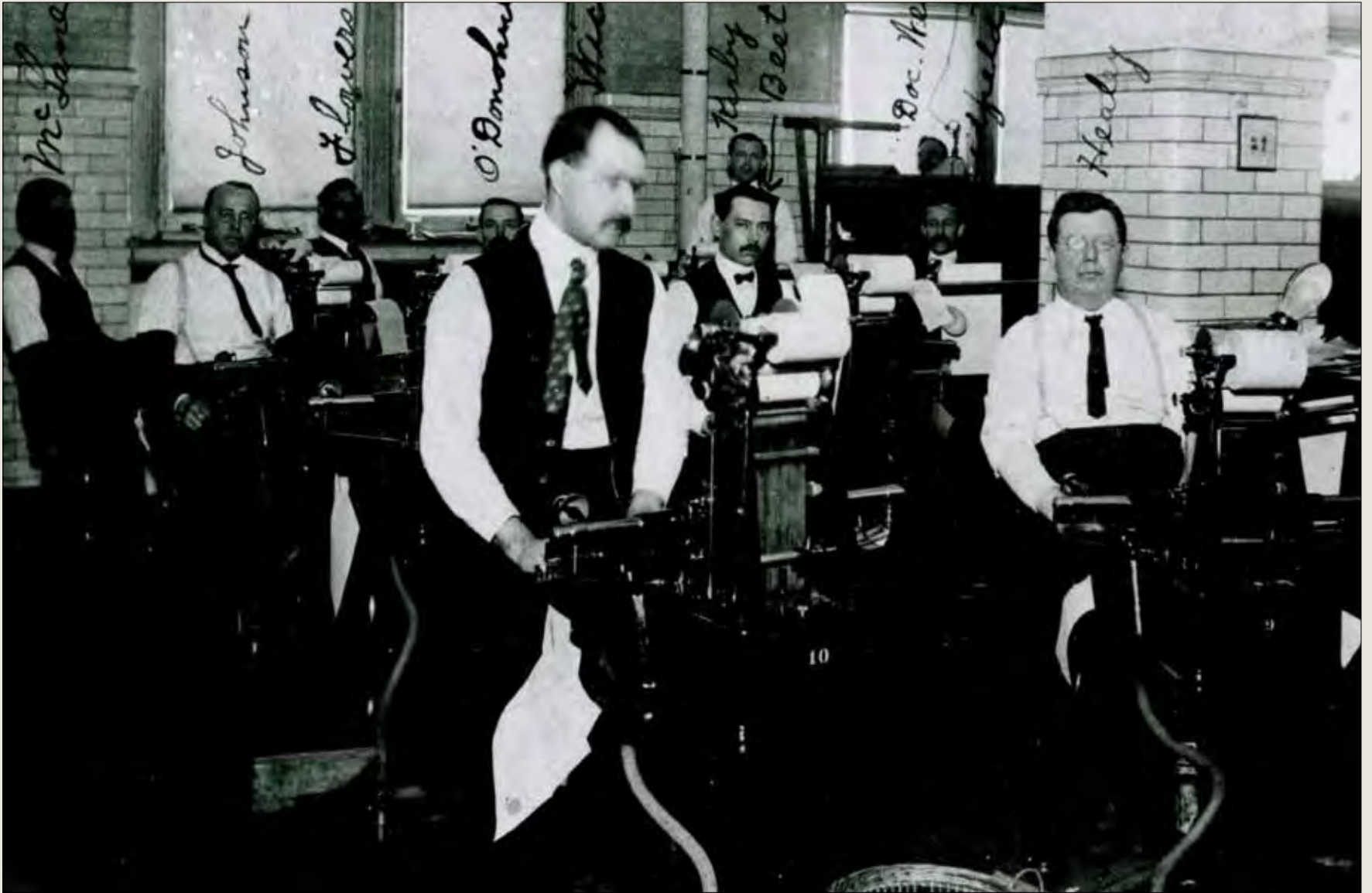
In 1904, the two most successful systems for setting type by machine were introduced to GPO: Monotype and Linotype. Monotype, which cast individual characters in metal, arrived with 28 machines “on trial.” This photo shows 10 of the first Monotype operators, journeymen originally trained as hand compositors.
