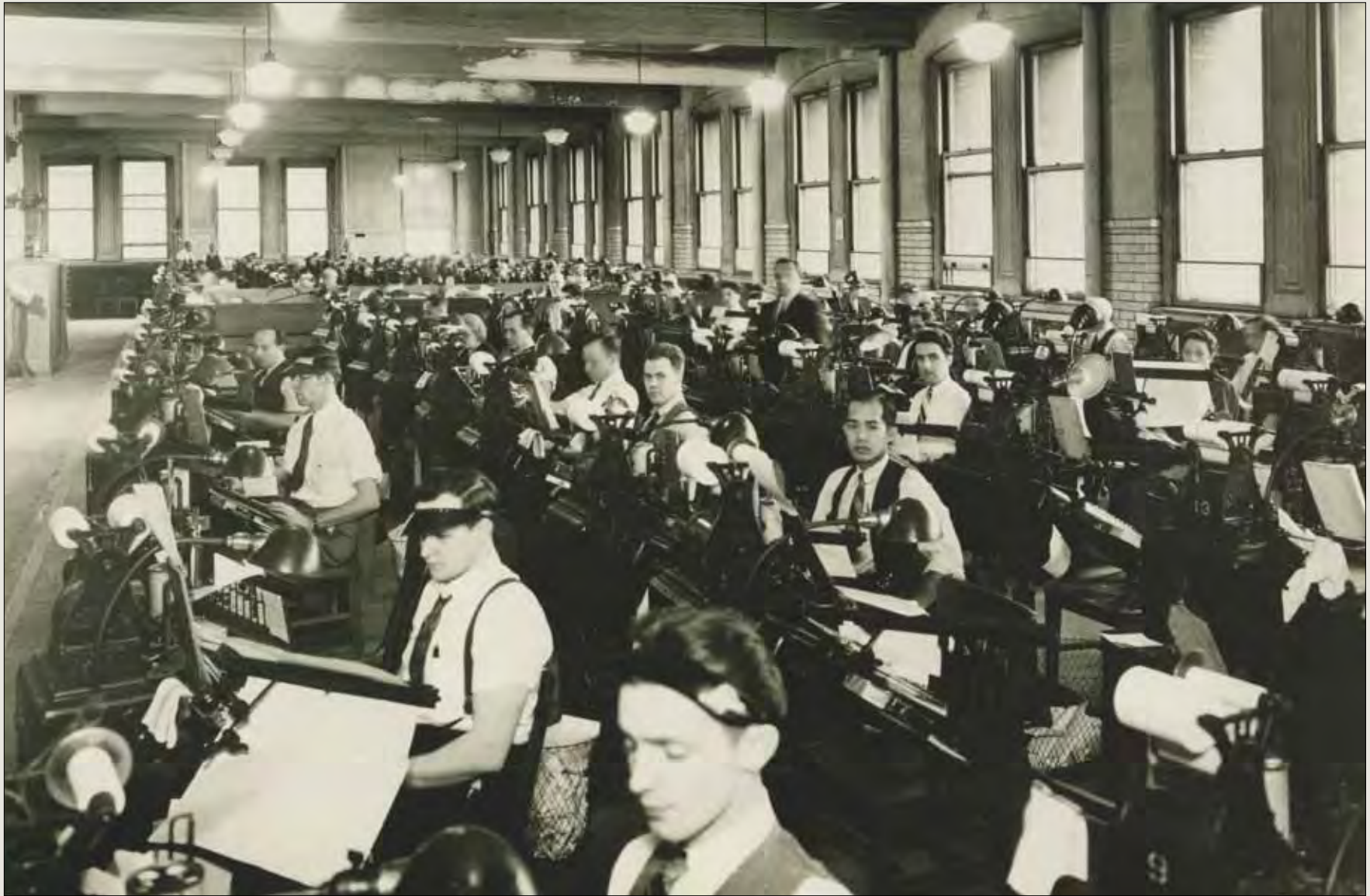
Monotype battery, circa 1930. Machine typesetting was an immediate success at GPO. From the original 28 Monotypes in 1904, the battery rapidly grew to over 100 by 1920. In 1916, the Lanston Monotype Company was boasting “the largest battery in the world” in its print ads. At that time two-thirds of all the type set at GPO was Monotype.
