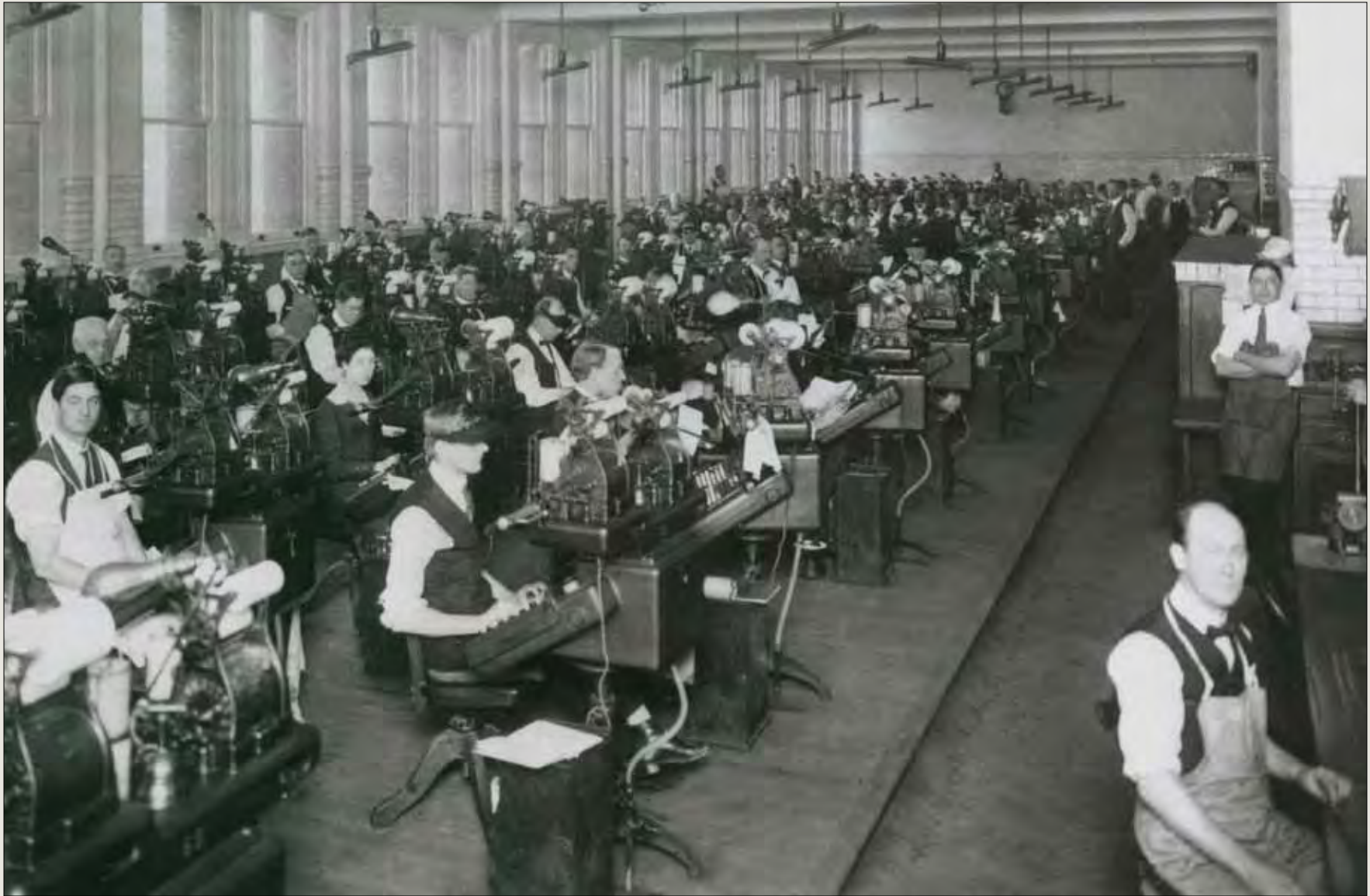
The GPO Monotype section was remarkable in many ways, starting with its sheer size, 120 keyboards at the peak. The keyboards required no electricity, only compressed air to operate. Because Linotype operators sat next to a pot of molten type metal, the machine was thought “unsuitable” for women to operate. The Monotype section, on the other hand, had female keyboard operators. Keyboard operators were considered journeymen printers. Operators of the casting machines were not. Photo circa 1910.
