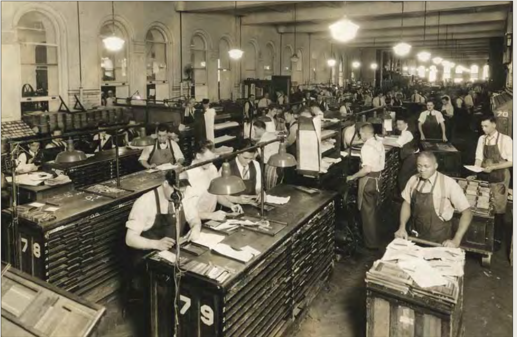
Compositors correcting Linotype galleys. Corrected lines were cast and substituted for flawed ones. Photo circa 1930.
