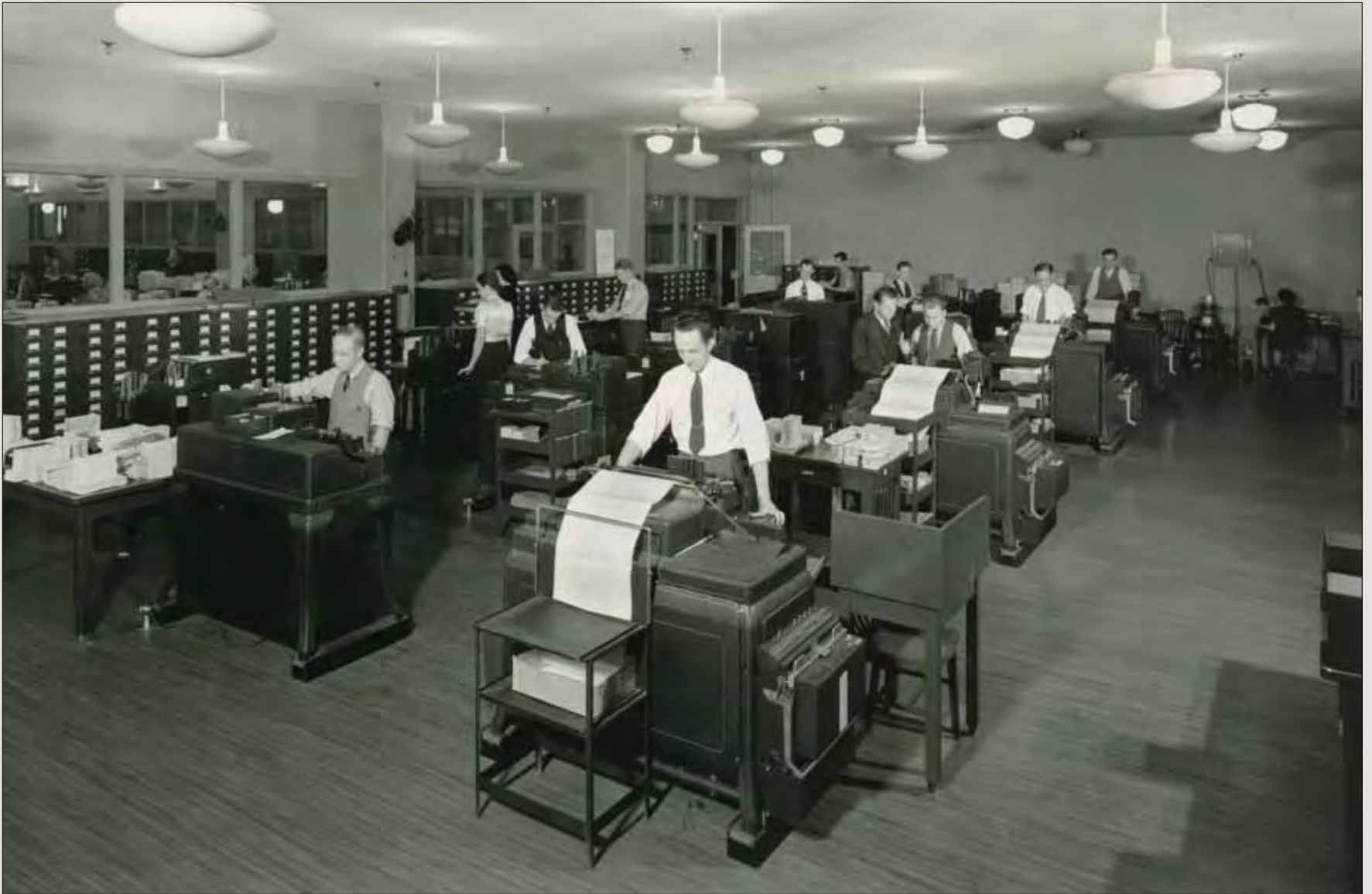
These machines read and tallied the punched tabulating cards during the 1940s. Although used throughout the Government and the business world, the first extensive use of tabulating machines was for the U.S. Census. GPO produced the tabulating cards.
