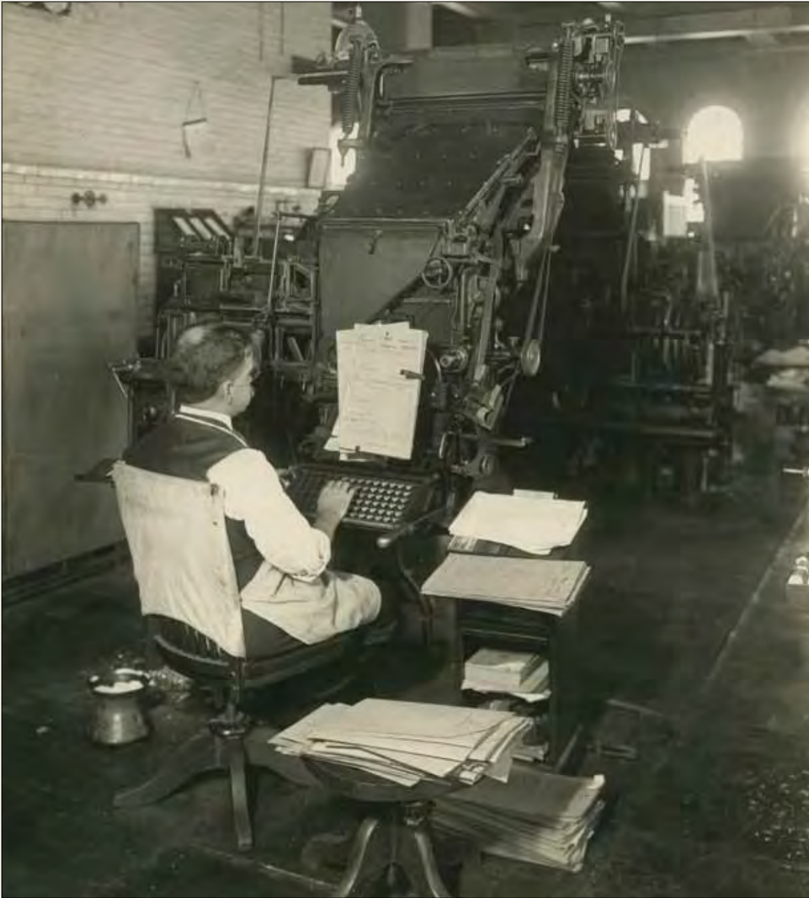
The Linotype, which produced a full line at a time (a “line o type” or slug) was well suited to so-called “straight work” — large unbroken blocks or columns of text. The Congressional Record , Federal Register , and U.S. patents were all big-volume Linotype products. Photo circa 1910.
