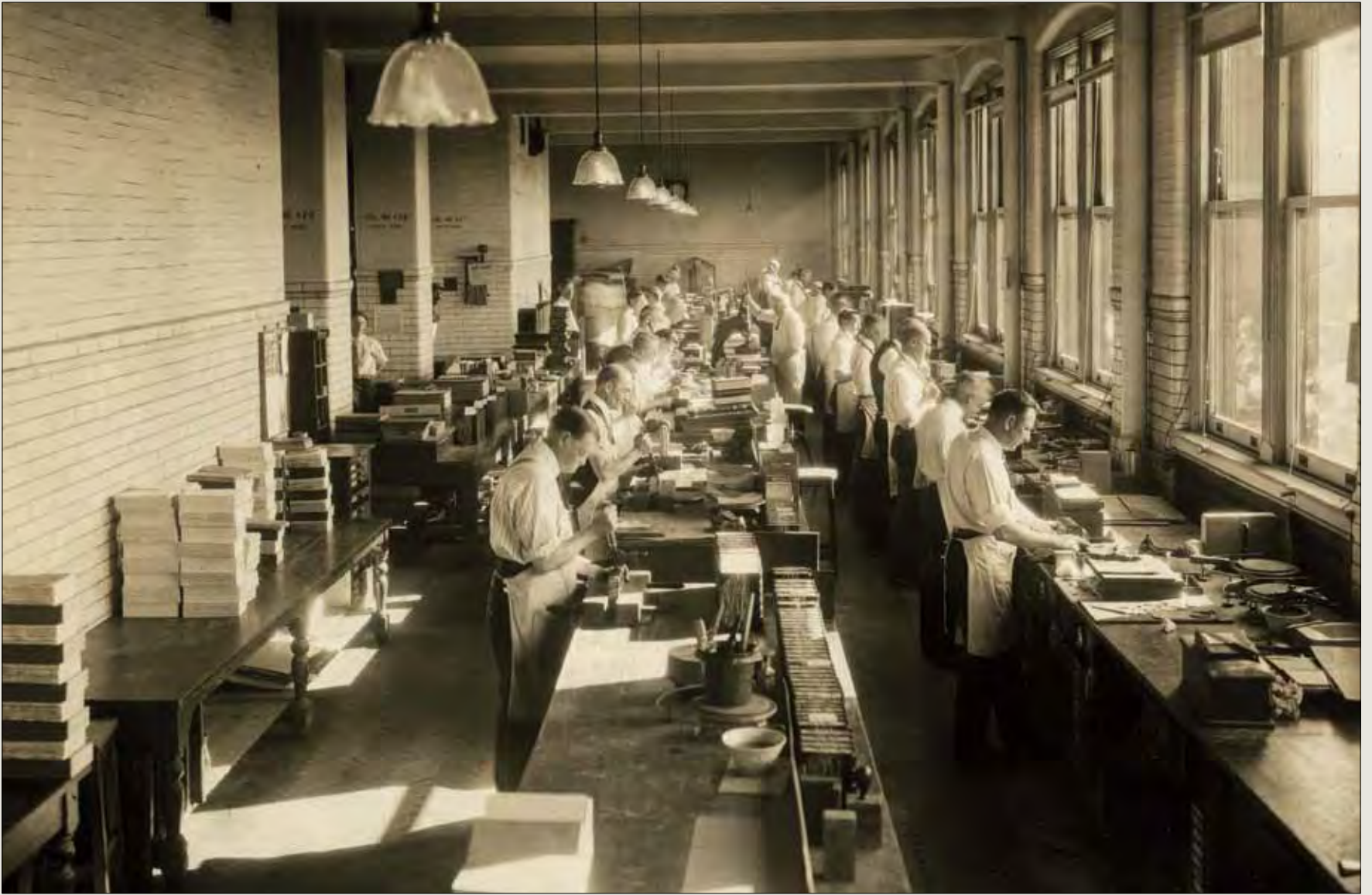
Bookbinders at work finishing cloth- or leather-bound books, circa 1905. Finishing involves stamping titles, other lettering, or decorative work on spines and covers.
