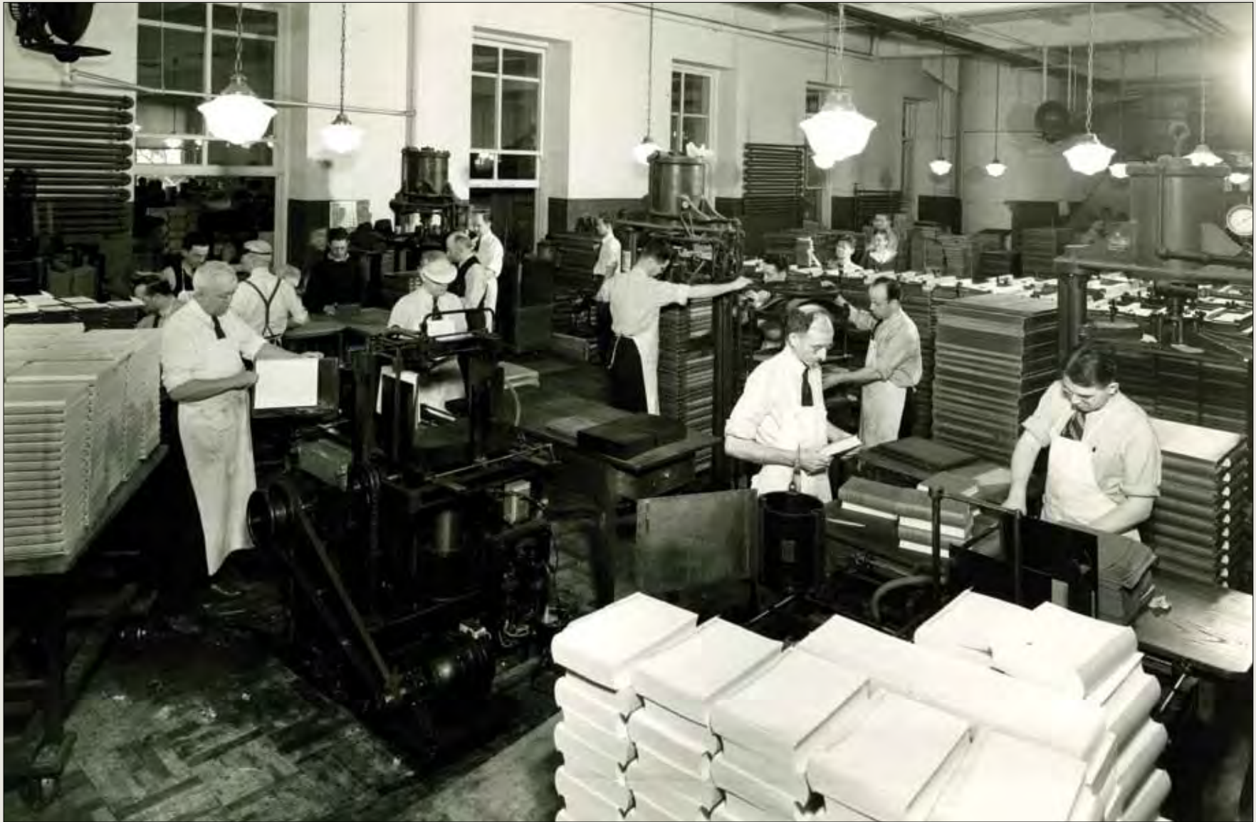
Bookbinding grew steadily more automated in the 20th century. In this photo from the 1930s, machines are used for making cloth-bound cases which are then secured to rounded and backed book blocks (shown here stacked in the foreground).
