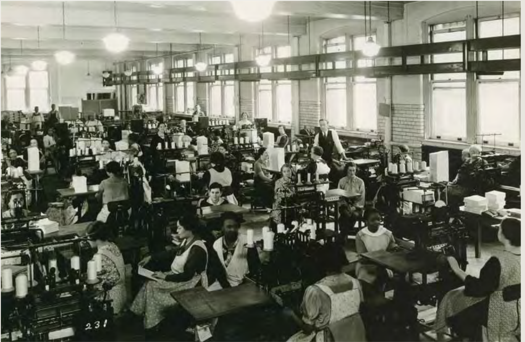
Daniel McConnel Smyth invented a machine for sewing book blocks for high-quality bindings in 1879. GPO adopted the machines almost immediately and ran an extremely large battery, as seen in this photo from the 1930s. Smyth sewing is still used today.
