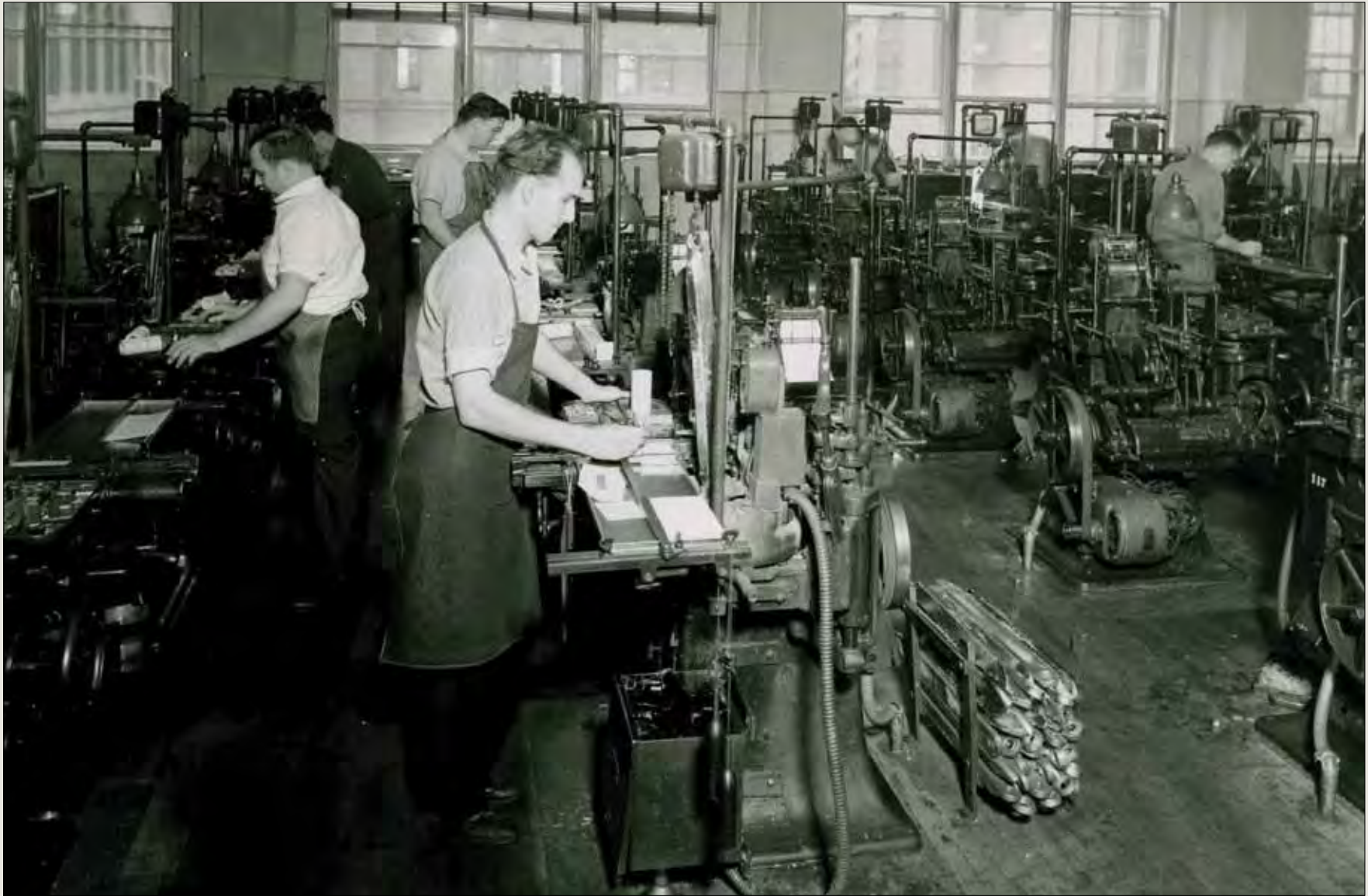
That ribbon was then read, employing compressed air much like a player piano roll, by the casting machine which interpreted the punches to guide a mold or “matrix” into position for metal to be injected to form individual letters of type, or “sorts.” Photo circa 1940.
