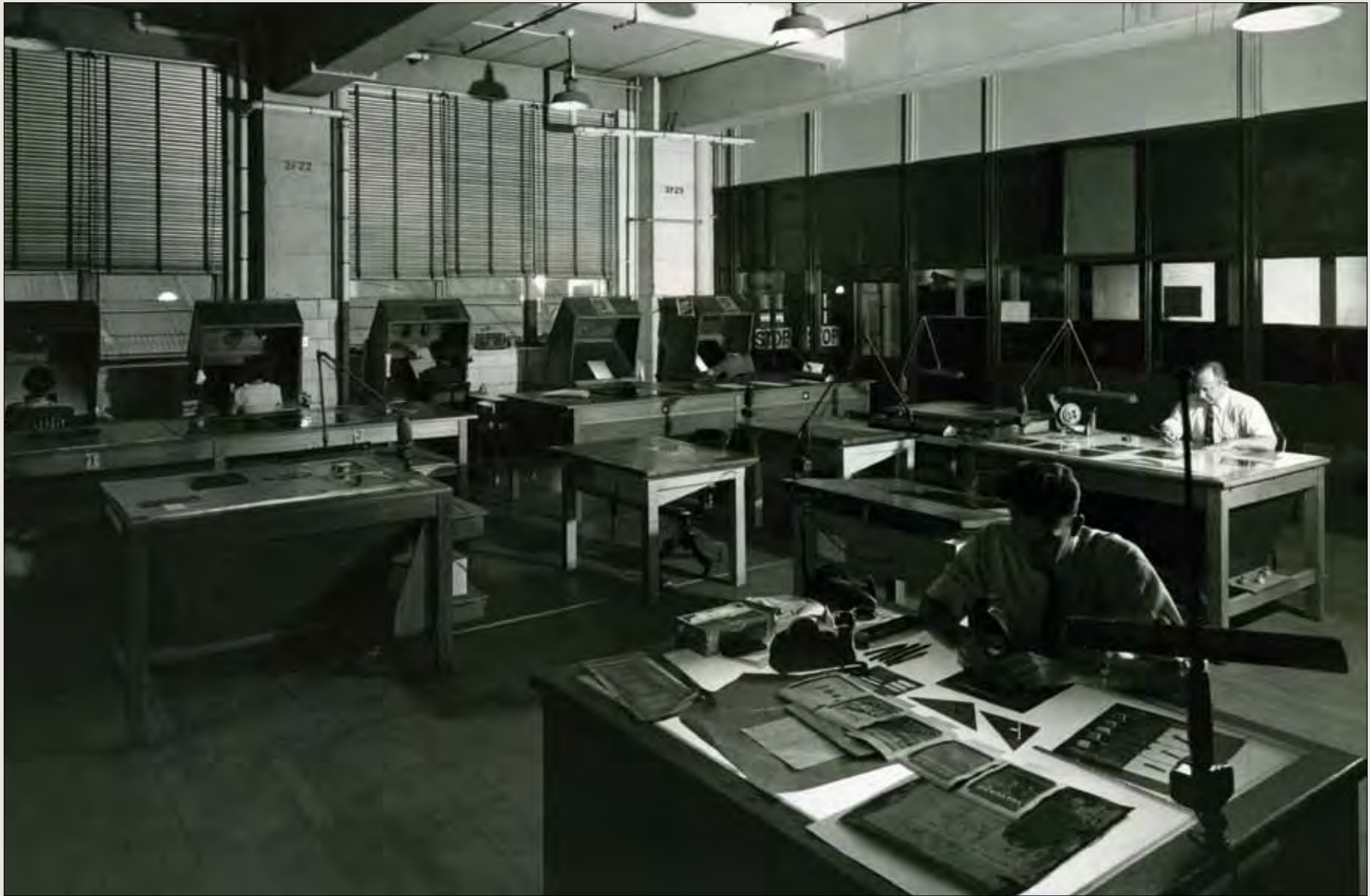
Offset was a photographic process. The page forms were prepared from photographic negatives, which were assembled by special compositors called Negative Strippers, seen at work here in the 1950s.
