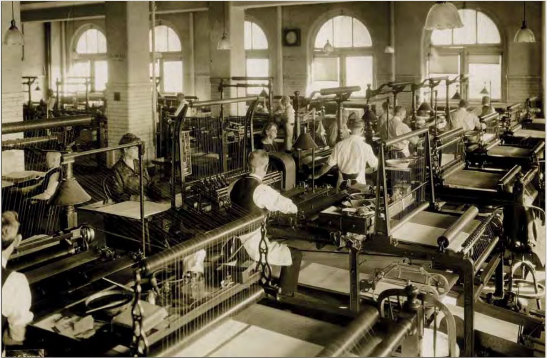
Ruling machines applied pale blue and red lines to sheets of paper for use in lined tablets and record books in this photo from the 1920s.
