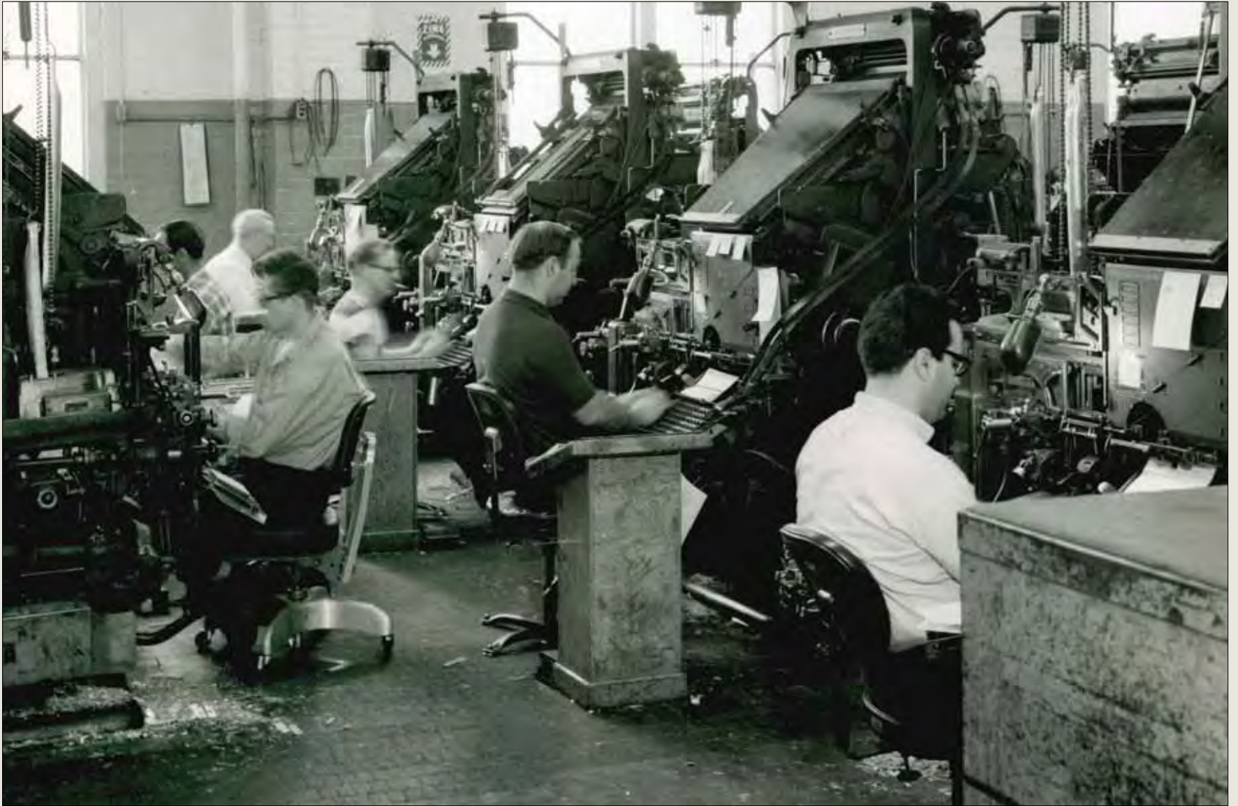
By the 1960s, although offset printing and phototypesetting had made inroads, hot metal was still king. GPO's battery was a mix of machines made by the Mergenthaler Linotype Company and the Harris Intertype Company. The four machines at the right of this 1970s photo are Intertypes, favored by some operators for their easier loading system for magazines of matrices.
