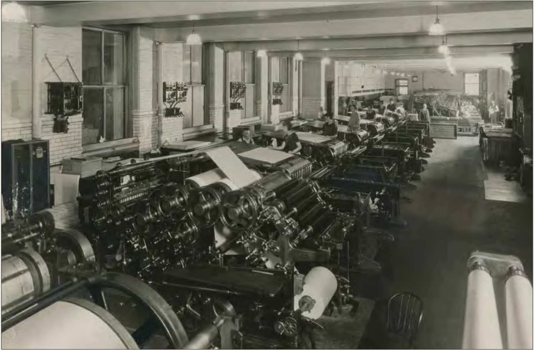
As GPO grew in the early 20th century, the diversity of work, thus the diversity of presses, grew steadily. In this 1920s view, at least three types of press are visible — web cylinder presses in the foreground, sheet-fed cylinder presses, and the sheet-fed presses known as “bobtails” in the distance.
