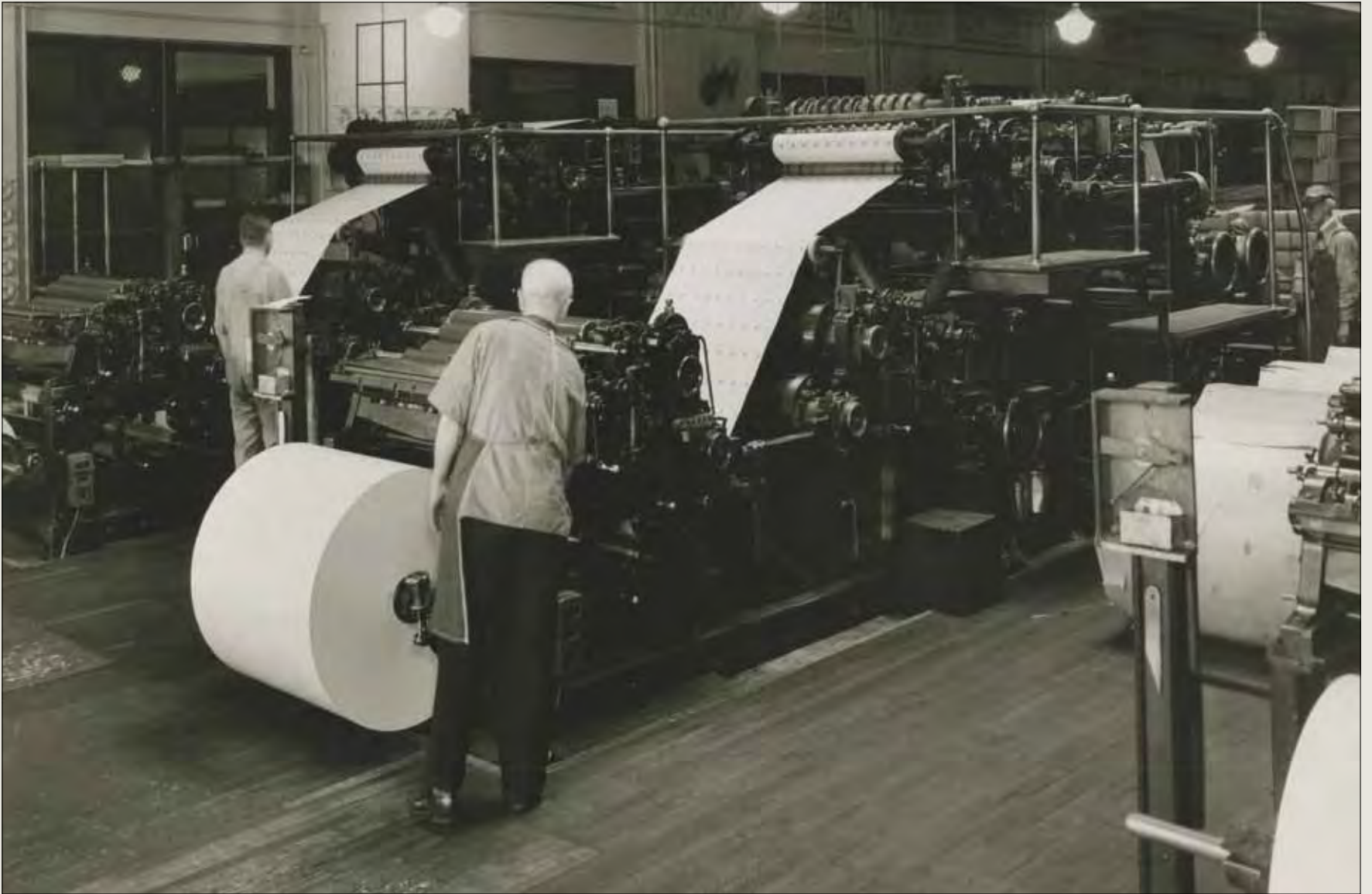
These presses printed money orders for the Post Office Department in Building 4, about 1950.
