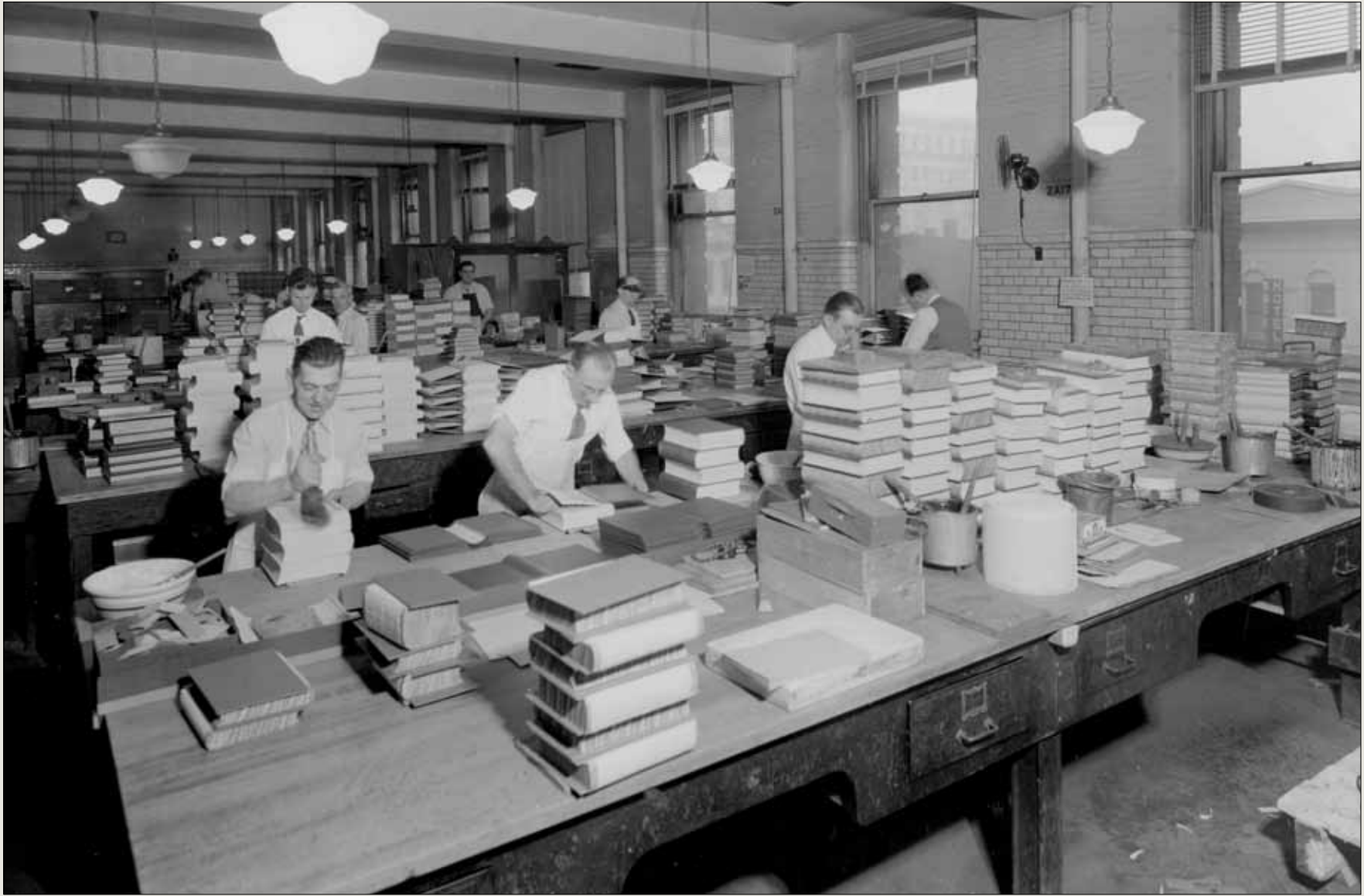
Bookbinders during the 1940s securing prepared text blocks in cloth-covered cases, or "casing-in."
