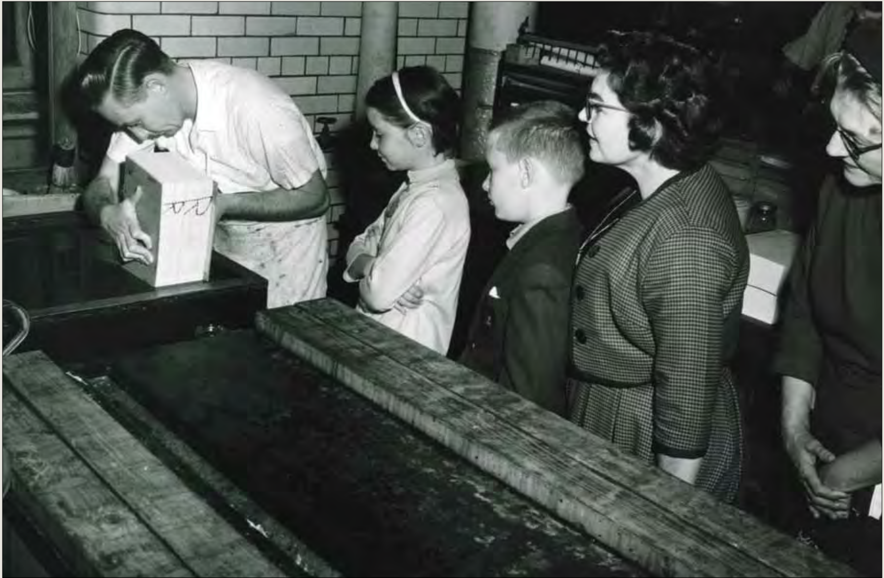
A GPO bookbinder in this photo from the 1960s, demonstrates edge marbling, where a decorative pattern is applied to the edges of a bound book by touching it to colored pigments suspended in a gelatinous medium. GPO has produced its own marbling since World War I, and continues the craft today.
