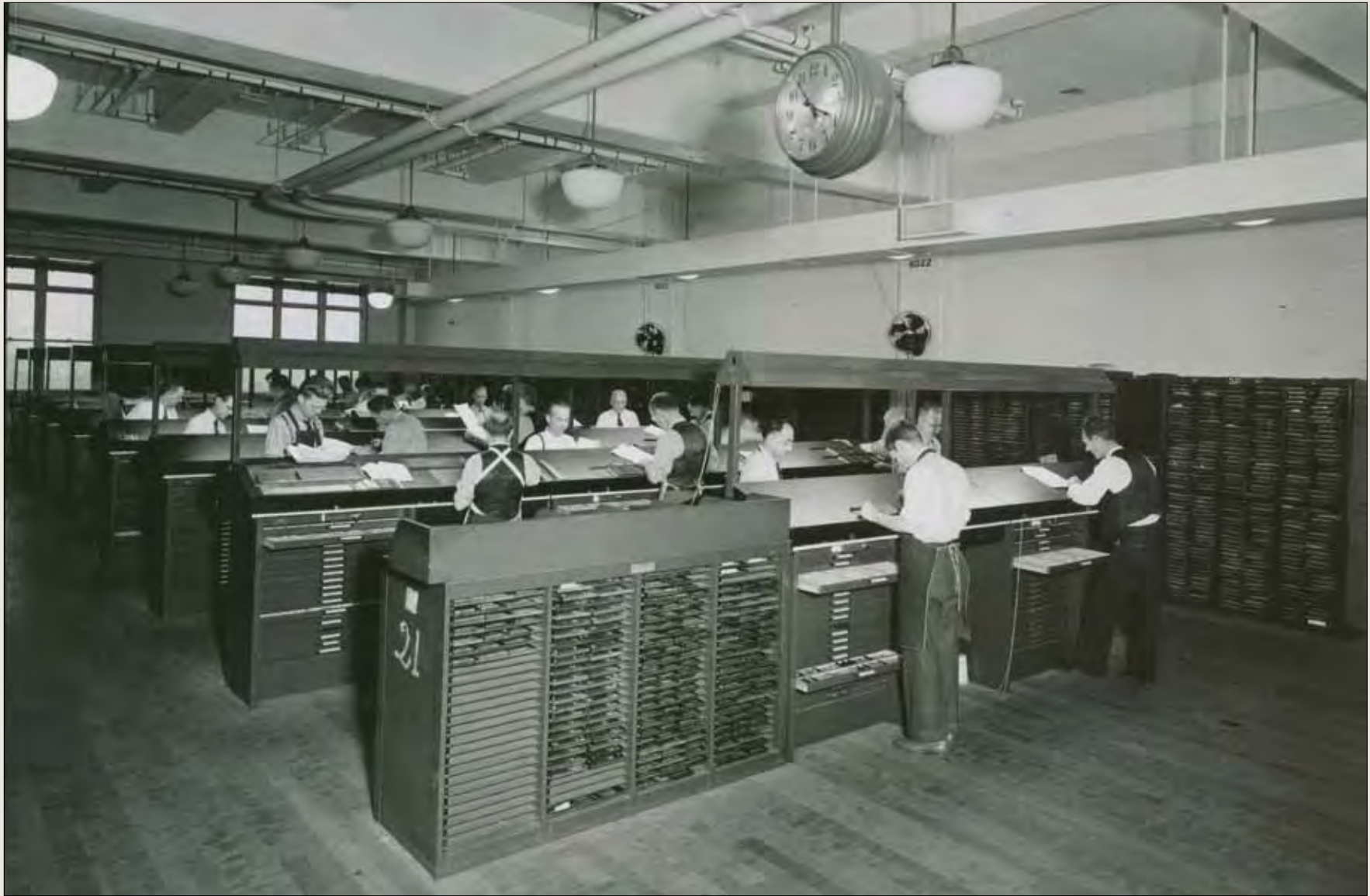
Compositors correcting galleys, probably Monotype. Once the proof was read and marked up, errors would be corrected by pulling the incorrect letters (“sorts”) from the galley and inserting the correct ones. For Linotype, the entire line had to be recast. Photo circa 1950.
