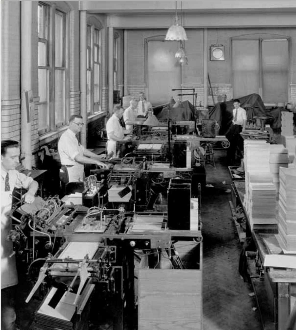
Machines that fabricate a cloth-covered board case came into wide use around the turn of the 20th century. Here four bookbinders operate casemaking machines in the 1940s.
