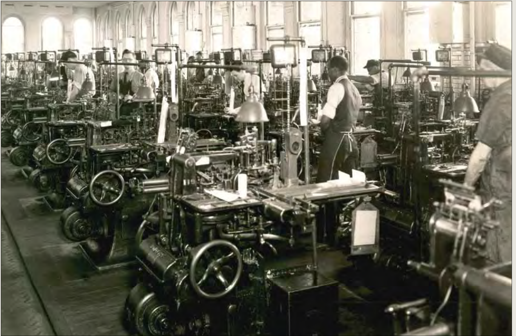
Casters could be set up for composition (producing galleys of sorts, properly spaced) or for sorts (producing letters, punctuation, etc.) that could be inserted by hand to correct mistakes in galleys). Photo circa 1930.
