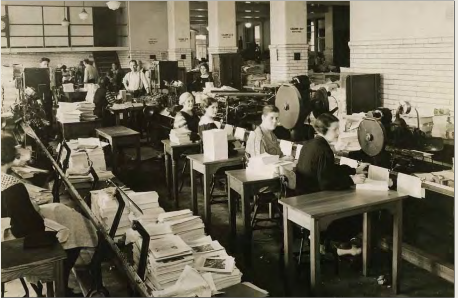
Among the many types of bindings GPO produced was a single section of folded sheets, secured into a pamphlet with a wire “stitch” (similar to a staple). Here, workers are shown on a pamphlet binding line in the 1930s.
