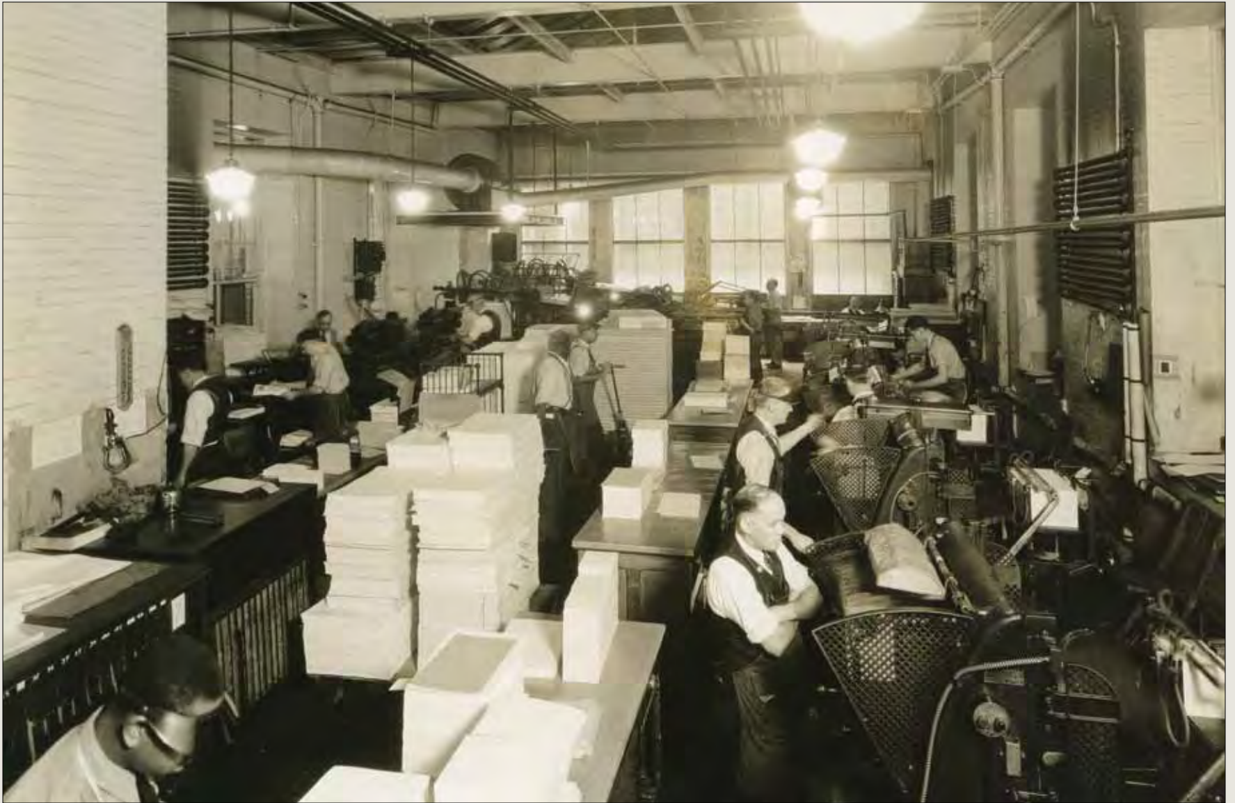
Machines for folding large quantities of paper were invented in the mid-19th century. Here, folding machines are being operated in the 1930s.
