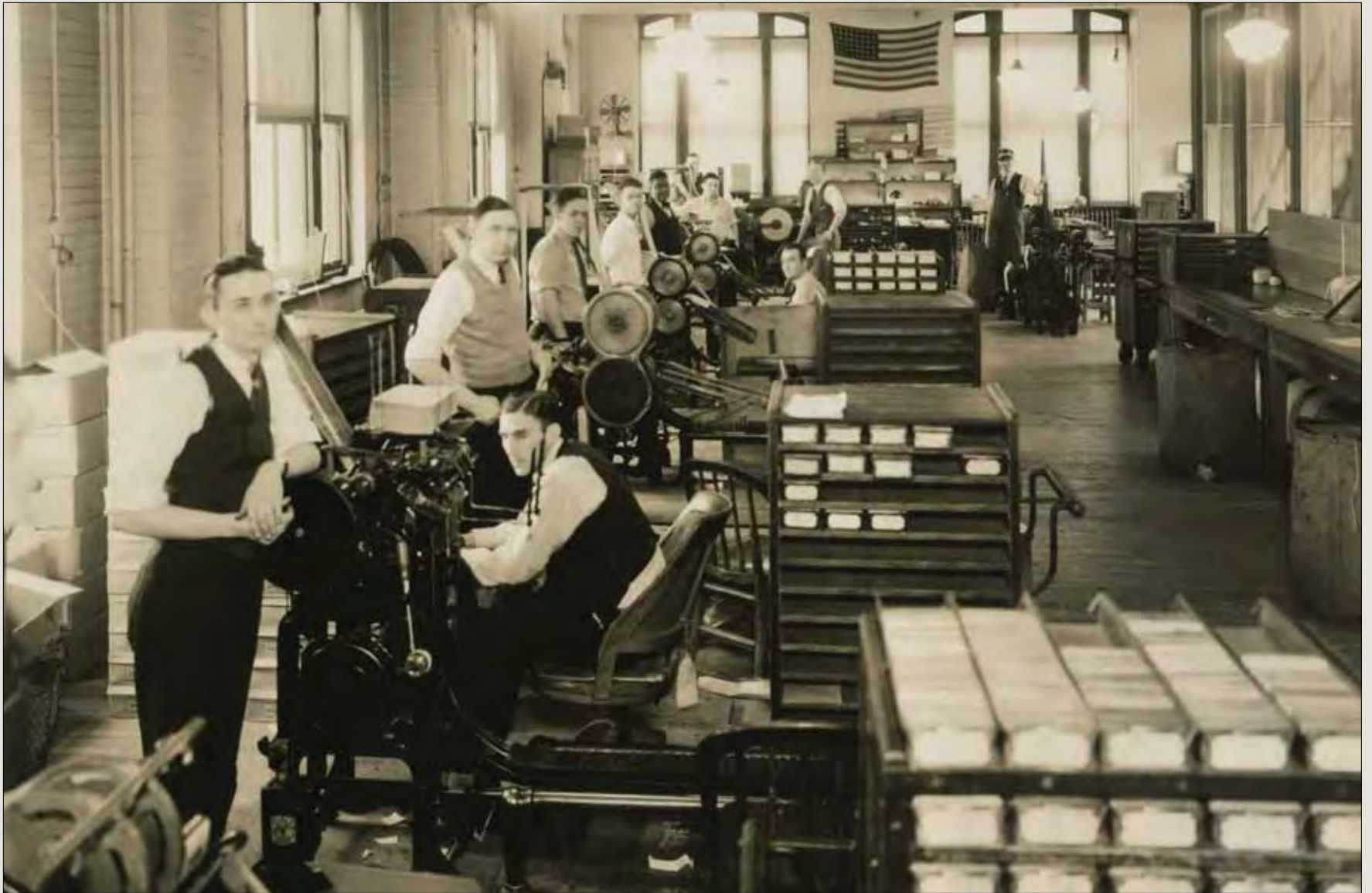
Like many large printing shops, GPO produced many products that were distributed by mail to individual subscribers, either on Capitol Hill, in Federal agencies, or elsewhere. In this photo taken during the 1930s, machines using Addressograph plates are used for direct-mail addressing.
