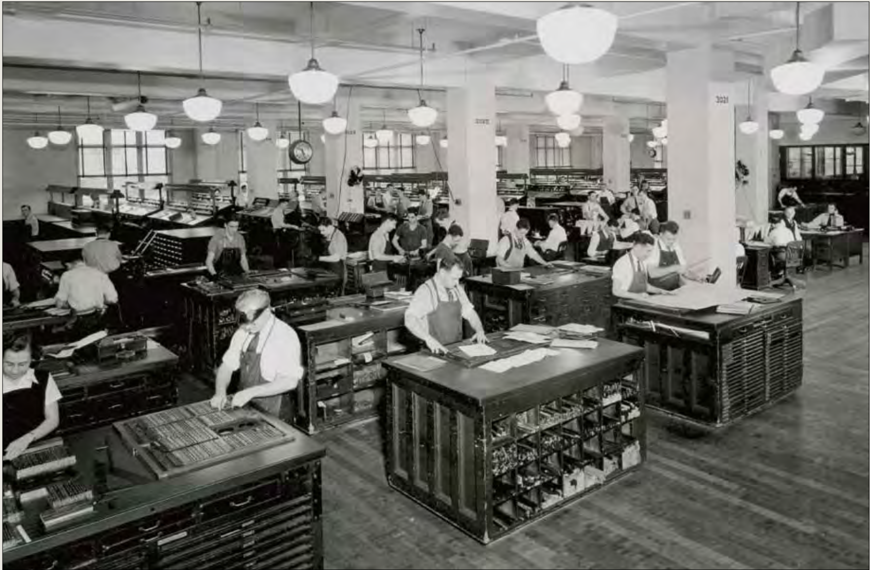
Once corrected, the galley type was made up into page form, a process known as “imposing.” Here compositors are at work at stone-topped tables imposing page forms in frames called “chases.” Chases could be taken directly to the bed of the press, although in most cases at GPO, a series of plates, which exactly duplicated the set and imposed type, were struck. A further set of “page proofs” was often taken and checked before plates were struck. Photo circa 1930.
