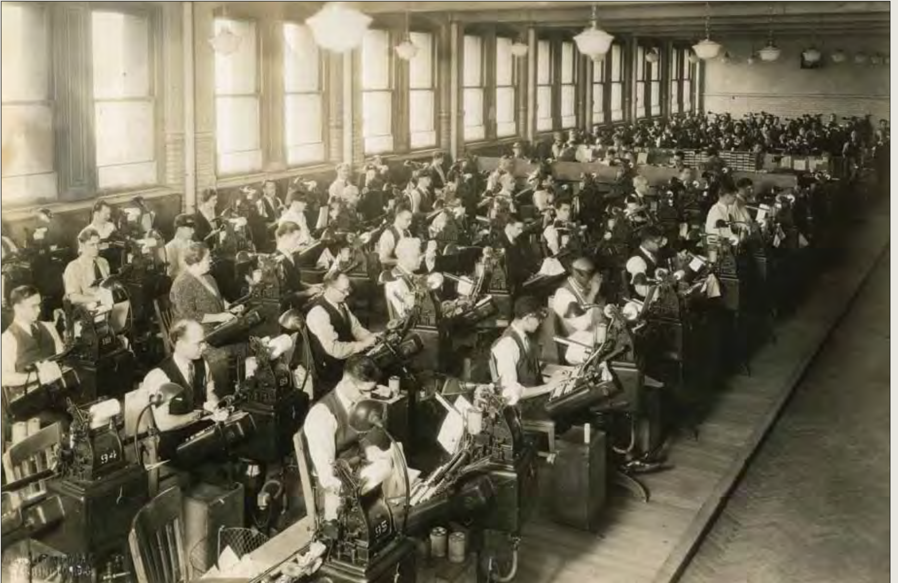
Monotype was a two-step system, as shown in this photo from the 1930s and the following. These operators typed copy on the keyboard which punched holes on a grid into a 4 1/2" inch wide paper ribbon. Their typing included letters, punctuation, and spacing, all of which was translated into the coded punches on the ribbon.
