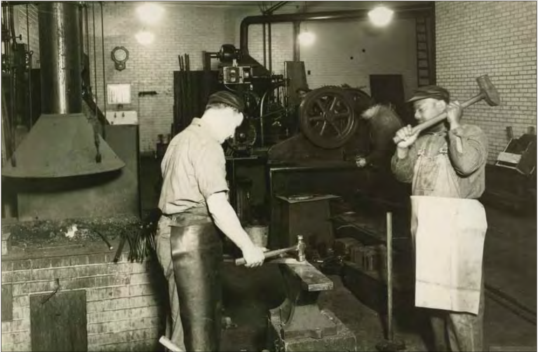
Many machine parts and repairs could be economically made by GPO's blacksmiths in the Metal and Pipe Section. In an earlier day, blacksmiths also kept GPO's delivery fleet working, shoeing the horses that pulled delivery wagons. Photo circa 1930.
