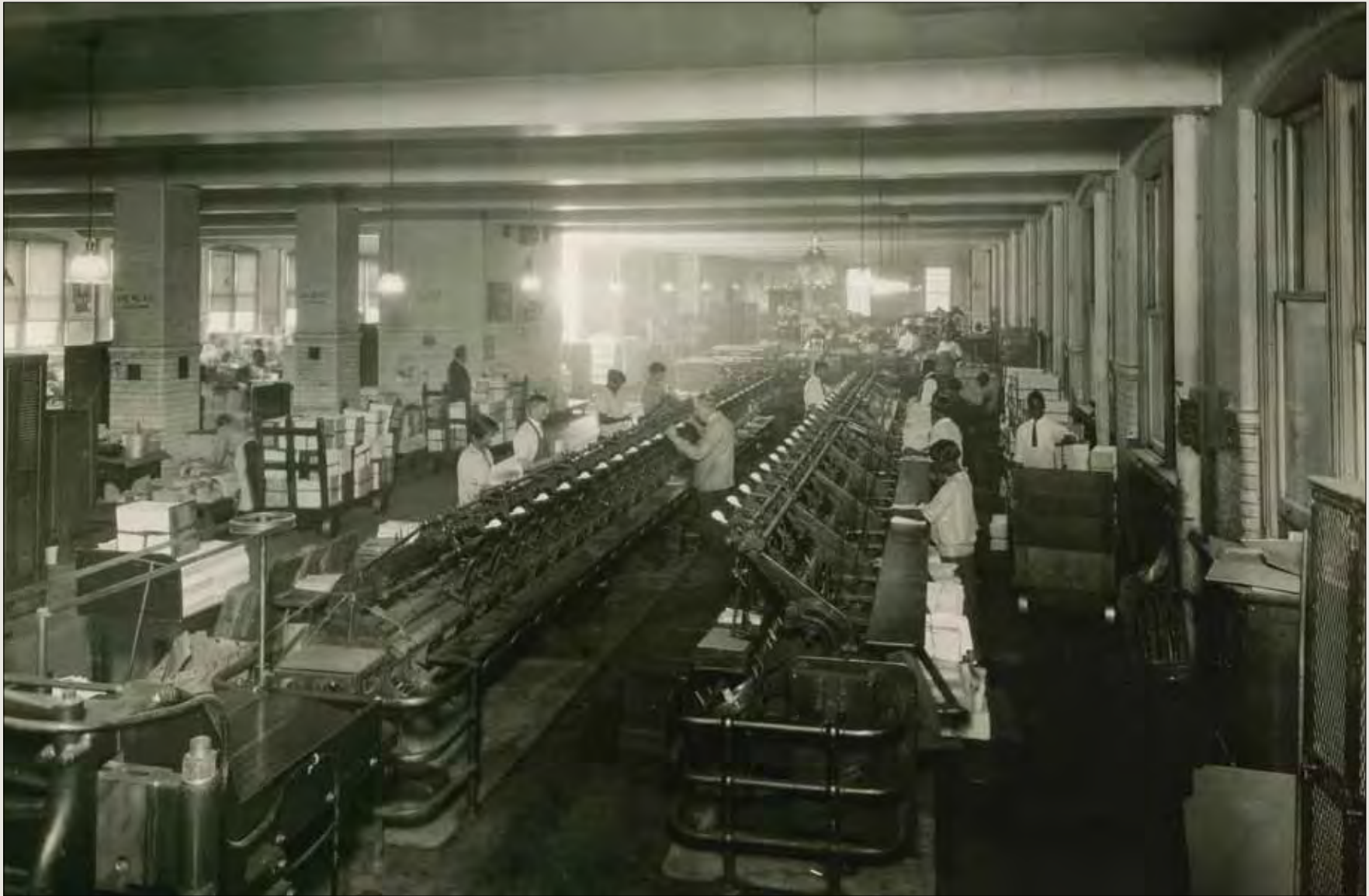
GPO's binders produced every kind of folded, stitched, sewn, or glued pamphlet and book. This production line made so-called "perfect bound" books and pamphlets, inexpensive bindings with a glued spine introduced to GPO around the time of this photo in the early 1930s.
