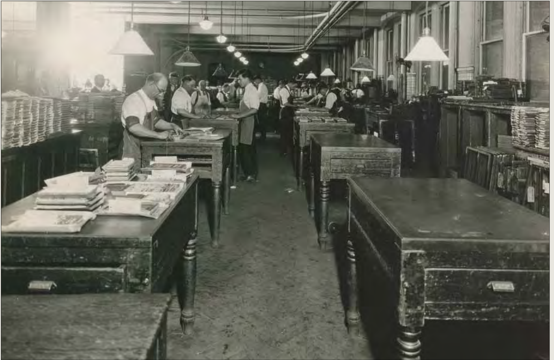
Type being assembled into galleys, about 1910. When complete, galleys were bound tightly with string.
