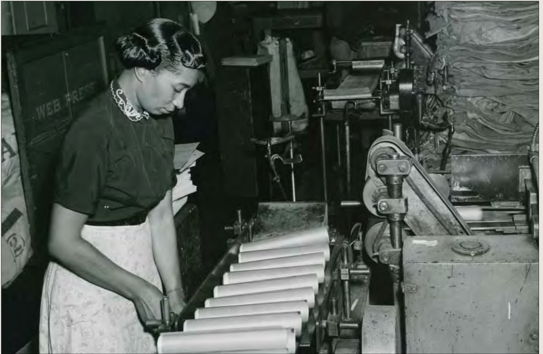
The capabilities of presses extended well beyond simply putting ink on paper. Presses could fold, emboss, score, or cut, and sometimes do simple stitched binding. This photo from the 1960s shows issues of either the Congressional Record or Federal Register coming off the press bundled, wrapped, and ready for mailing.
