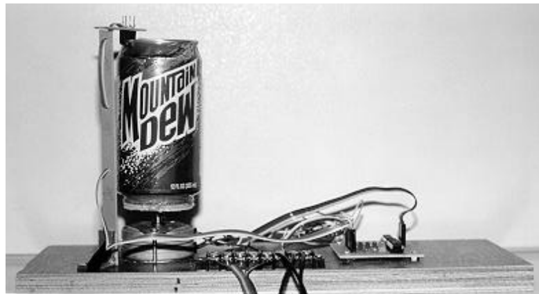
Figure 3: Soda-pop can version of stepper motor setup
