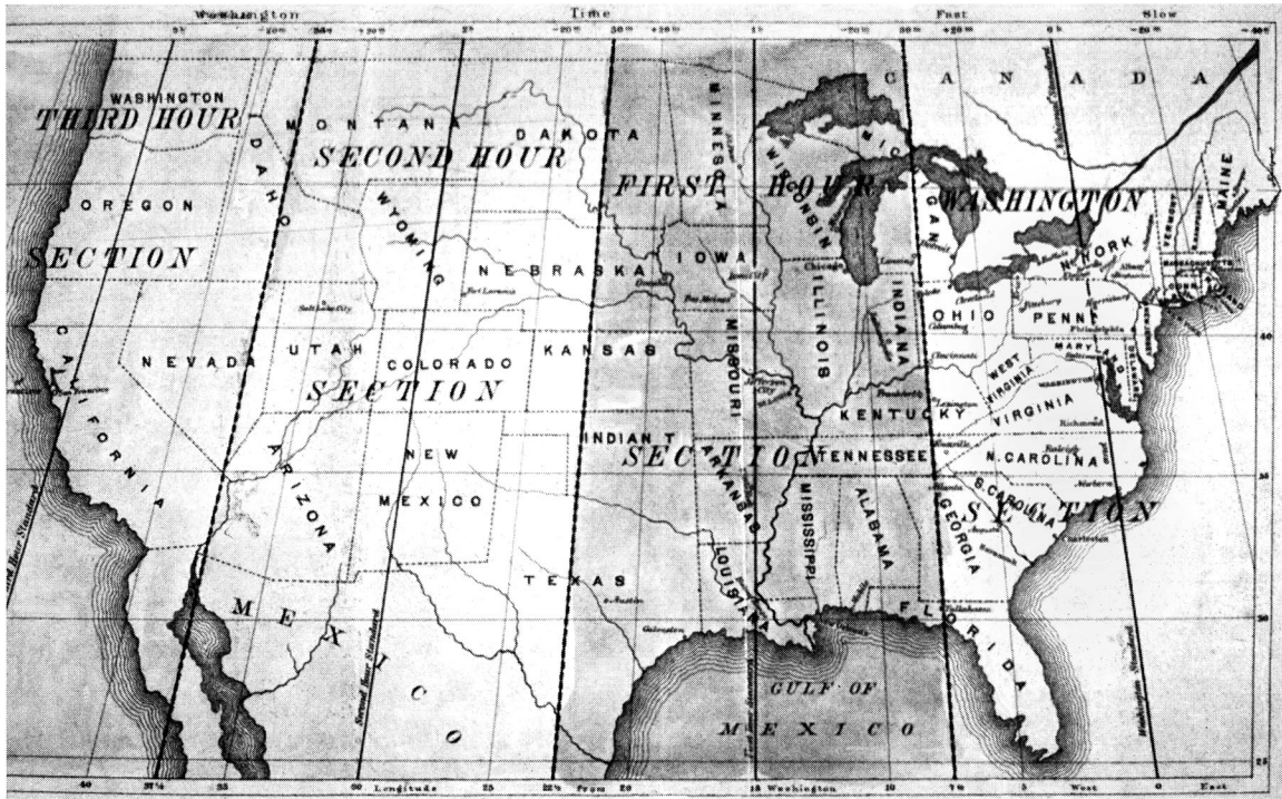
Figure 2. Dowd's 1870 map dividing the United States into four zones with precise longitudinal boundaries between the zones. The zones are indexed to the U.S. Naval Observatory's meridian in Washington D.C., not Greenwich, England. Sources: Dowd (1870) and Bartky (2000).
