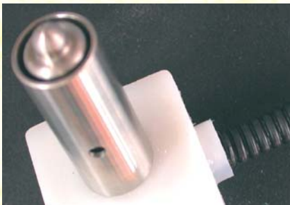
A-sample of the future series-type sensor with temperature measurement (and calibration curve) Source: VDI-Berichte (2003)
