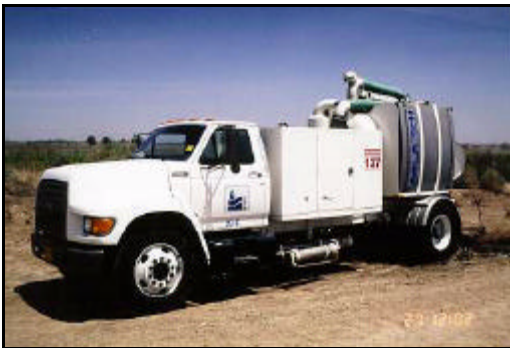
Figure 180: A sewer cleaning unit provided for use in the Mexicali effort by the U.S. (Apr 1995)
