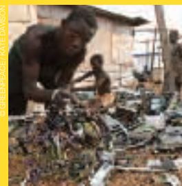
Boys breaking computer components in order to reclaim metals such as copper and aluminium. The cables are stripped or burnt to extract the copper.
