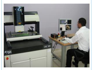
In addition and as a complement, thanks to the scanner function of the Smartscope, MEM provides engineering firms with the possibility to gather point clouds or the DFN of a component.
