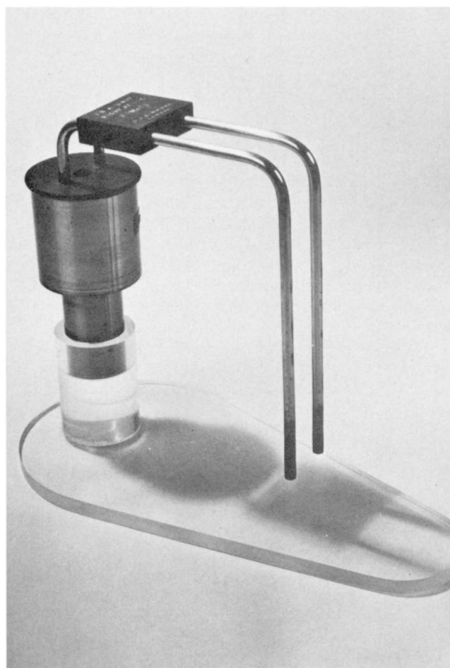
Fig. 15. B.A. standard of resistance. This standard resistor, constructed in 1863 and 1864, was the first electrical standard to be distributed widely. It consisted of a coil of platinum-silver wire wrapped in silk, imbedded in paraffin and enclosed in a thin brass case. The heavy leads were made of copper. In operation the standard was used in a water bath. Soon after it was introduced the "B.A. unit" became known as the "ohm." (National Bureau of Standards photo.)
