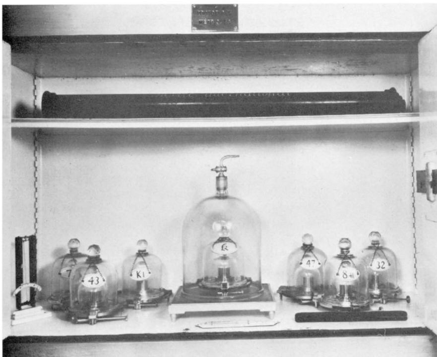
Fig. 8. Vault at the International Bureau of Weights and Measures. On the top shelf is the international prototype meter bar of 1889 in its protective case. On the bottom shelf is the international prototype kilogram, its six check standards, two thermometers (one of the maximum-minimum type), and a hygrometer. (International Bureau of Weights and Measures photo.)
