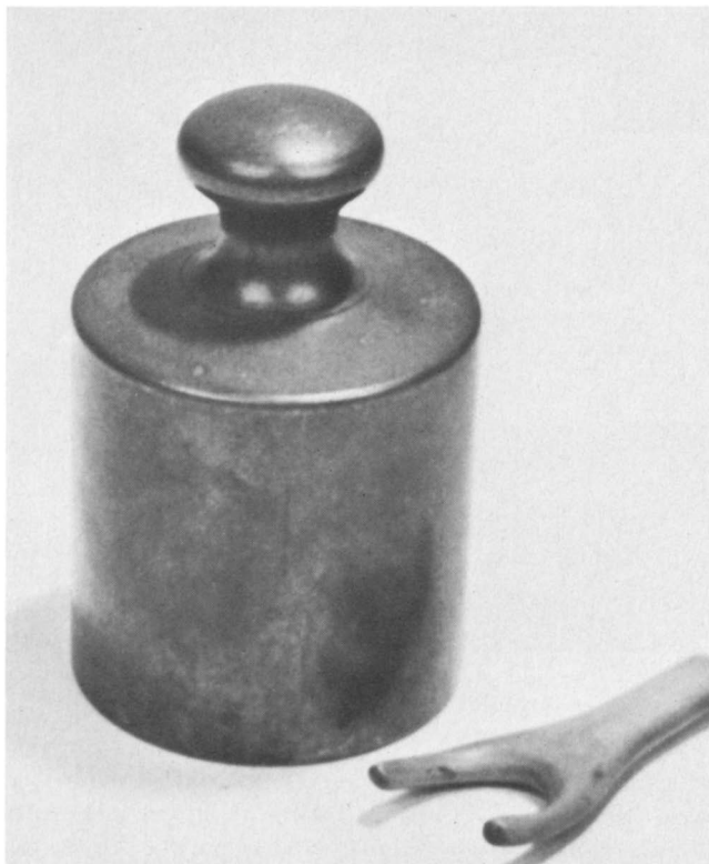
Fig. 3. The grave, a provisional standard of mass constructed in 1793. It was succeeded by the kilogram in 1795. (National Bureau of Standards photo.)
