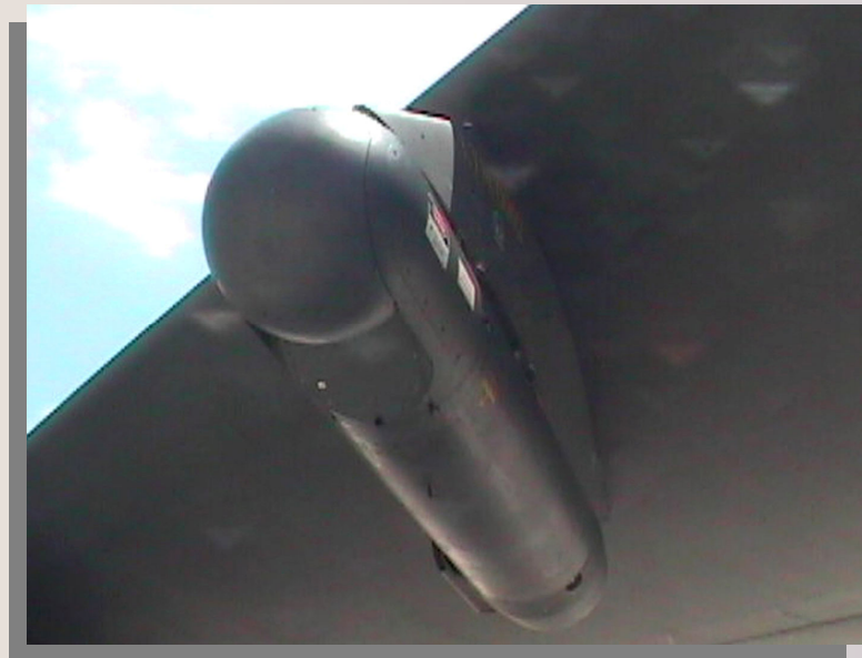
49th Test and Evaluation Squadron demos LITENING pod visual feed. A LITENING pod sits under the wing of a B-52 Stratofortress. The 49th Test and Evaluation Squadron's demonstration showed the B-52's LITENING pod's capability to capture digital imagery and upload it to communications networks. (U.S. Air Force photo)
