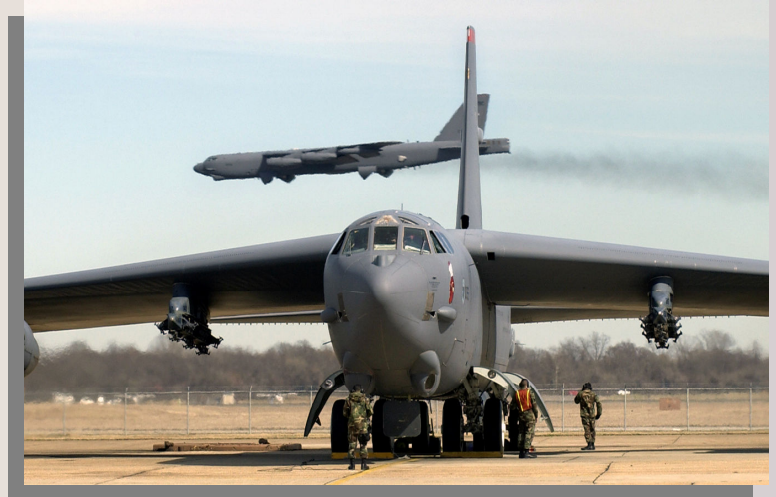
A B-52 prepares for departure as another B-52 arrives. The B-52 is capable of flying 8,800 miles without refueling and can carry a weapons load of up to 70,000 pounds. (U.S. Air Force photo/Tech. Sgt. Robert Horstman)
