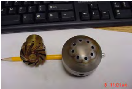
Taunton boiler "gun nozzle" after operation with B5 bioheat fuel blend, before cleaning
