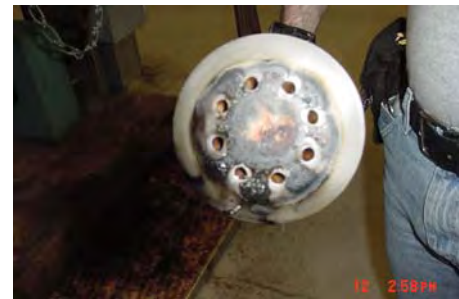
Taunton boiler "gun nozzle" after operation with #2 fuel oil, before cleaning
