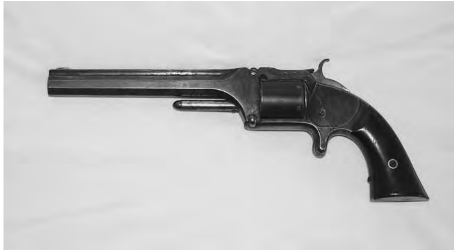
One of the two revolvers George Herrick “liberated” from a Confederate officer. The Smith & Wesson Number Two Army Tip-up is a .32-caliber six-shot revolver with a spur trigger (no trigger guard) and wood grip. The barrel tips up to remove the cylinder for loading. The shell ejector rod under the barrel is used to punch out fired cartridge cases one by one.
