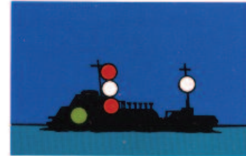
Vessel of less than 50 metres engaged in underwater work underway - by night
