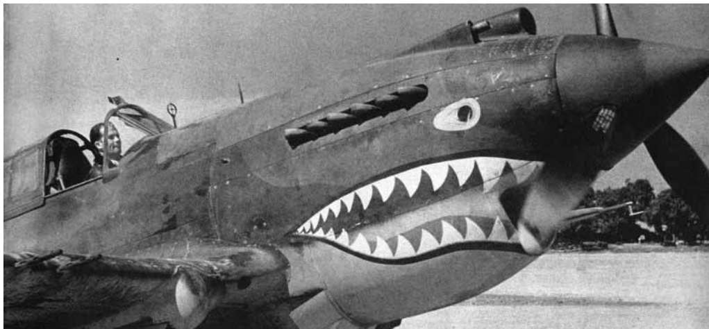
American volunteer group pilot takes his p-40 tomahawk off the field north of rangoon. Notice two guns on edge of each wing, one each side of cowlings.
