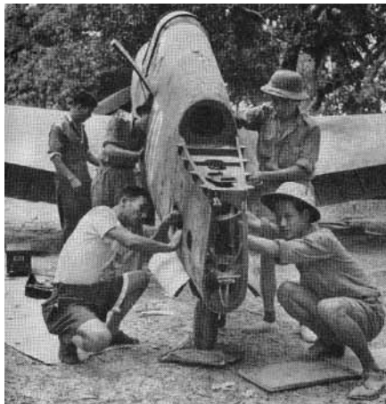
Chinese ground crew works on damaged tail of P-40. With hand tools they can make any part of a plane's body work. They consider association with A.V.G. a high honor.
