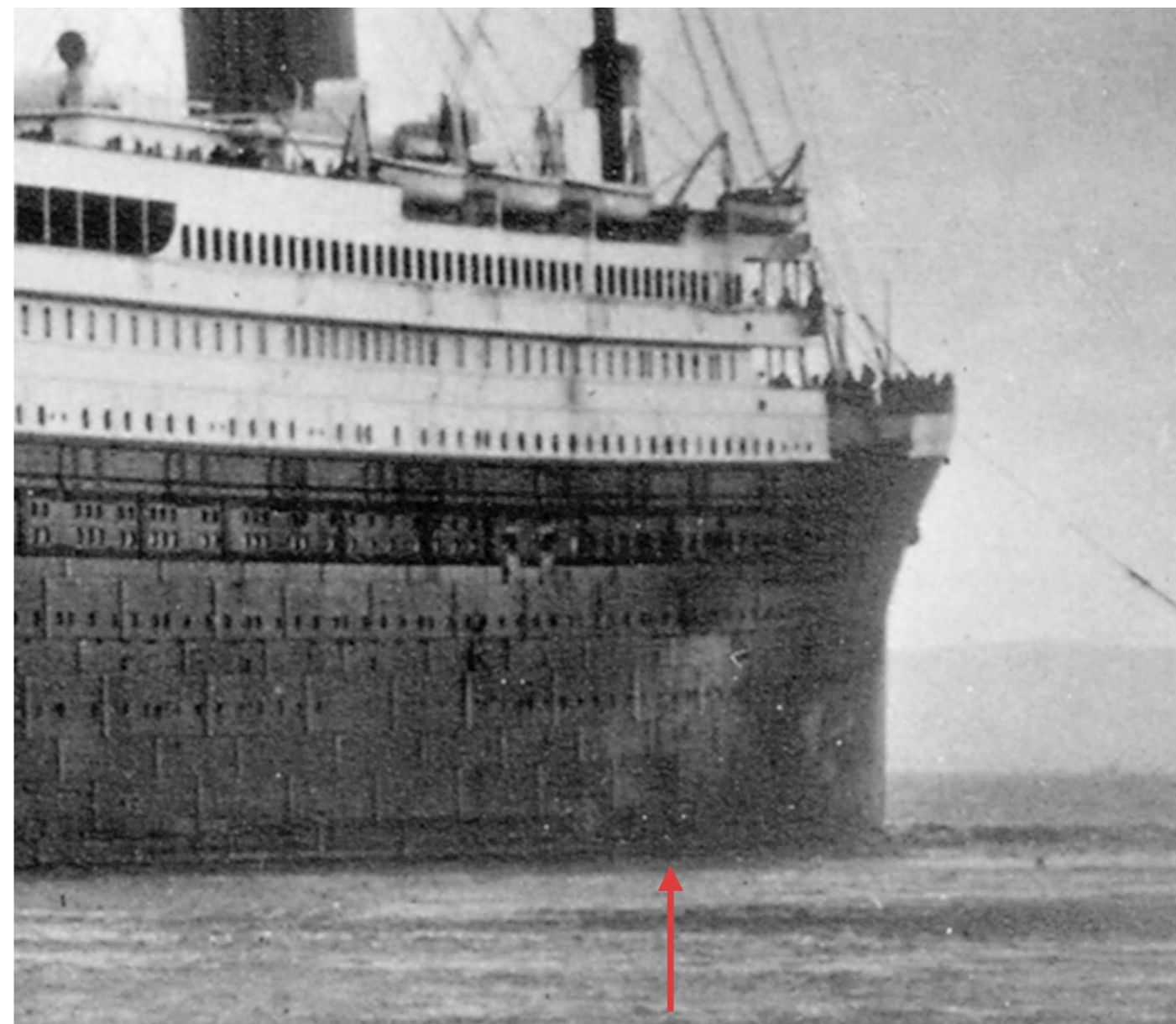
Above: This photograph also shows the Titanic as she departed Belfast on her trials, on 2 April. The angle from which the photo is taken is very different from that of the Kempster photos and the photo on the opposite page. The red arrow again shows the location of WTB E, yet there is no evidence of any hull deformation, only variations in tone from the patchwork paint job done to the ship's hull as she prepared for her maiden voyage and which was never perfectly completed. (Authors' Collection)
