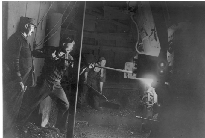
Stokers feed the furnaces on a coal-powered steamship, ca. 1898. (Library of Congress, Prints & Photographs Division)
