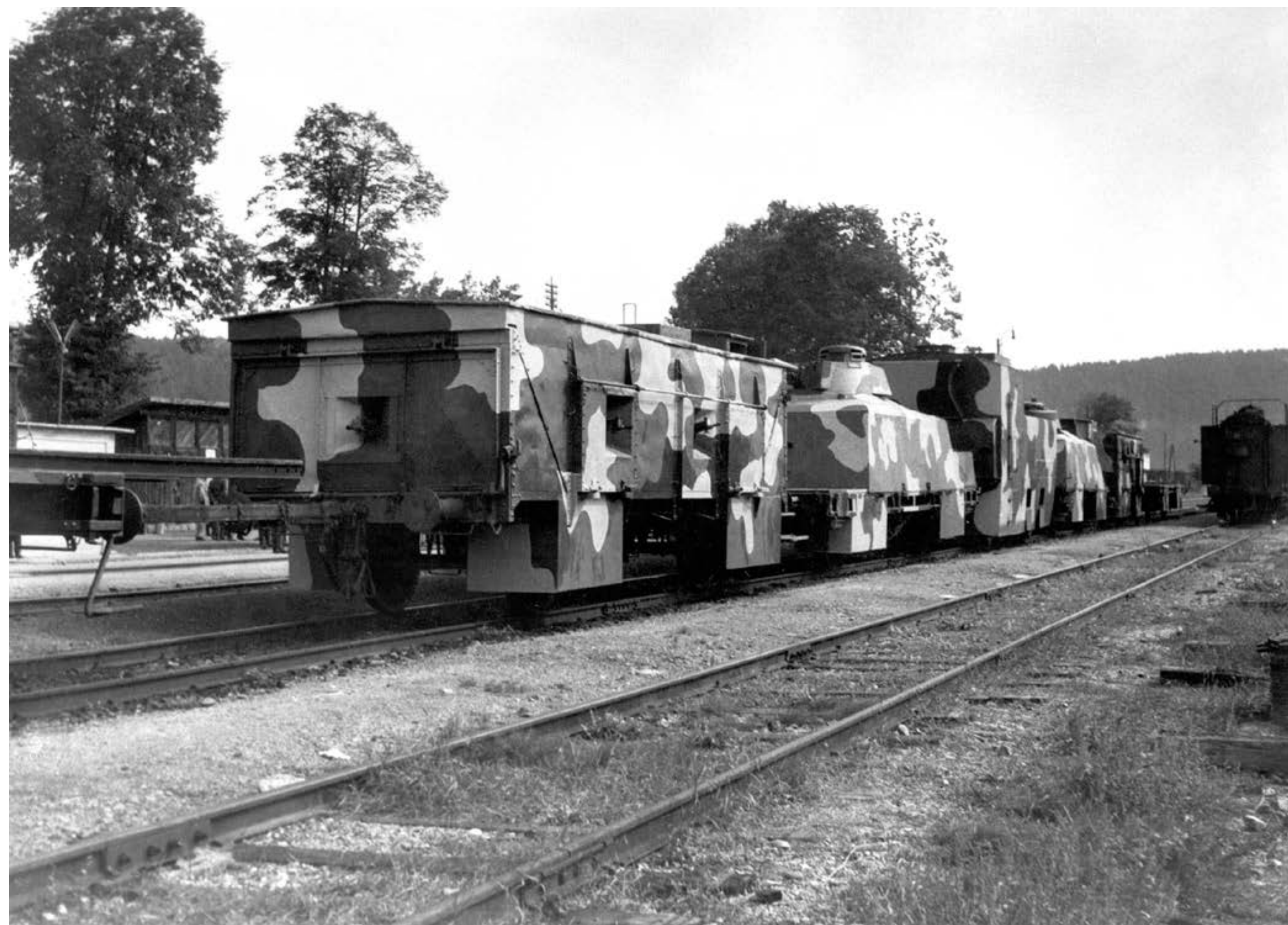
Armoured train – the Štefánik. Orders to start construction of the Štefánik armoured train had been issued by September 4, 1944. The trains were built in workshops belonging to the Slovak Railways in Zvolen. The first train was constructed in a record 14 days, the Hurban – the second armoured train – followed closely behind 11 days later. If we include a third train – the Masaryk – then the armoured trains were constructed in 5 weeks.
