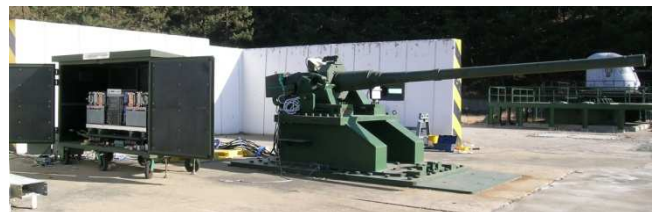
Fig. 14. Firing experiment of the ETC gun using the 150 kJ CCPPS
