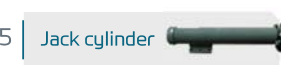
05 Jack cylinder Supports vehicle horizontally for accurate firing control using the hydraulic power from the main pump.
