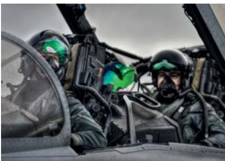
Communications & Control: Electronic Systems has developed the helmet-mounted display and targeting system for Typhoon. The Group's helmet technology is being adapted for the F-35.
