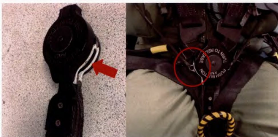
Figure 1.4.7 – ‘White whistle’ into which the lower lug of the AREL was fitted.
