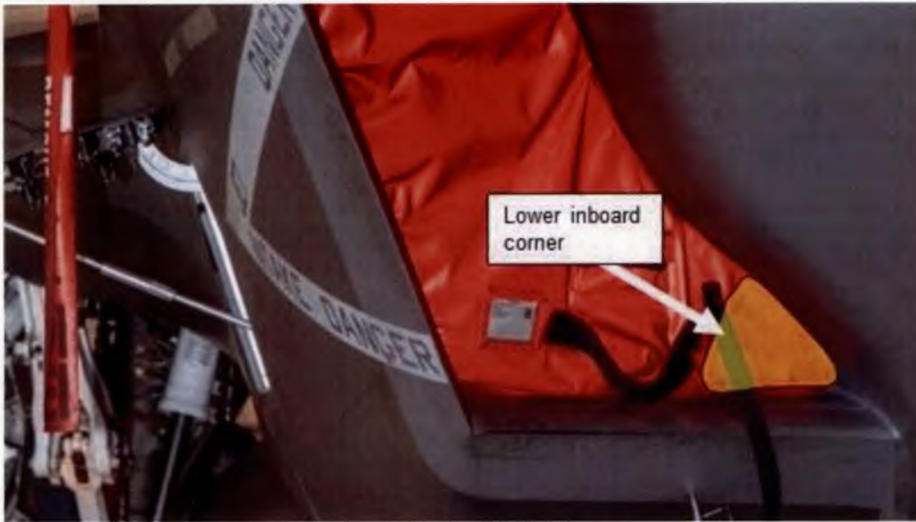
Figure 1.4.28 – Example of observed intake blank fitted to aircraft under maintenance, highlighting the inboard lower corner.
