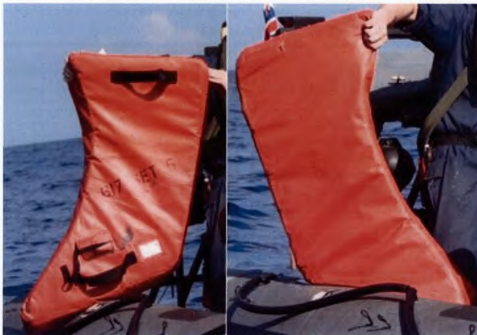
Figure 1.4.21 – BK-18 left intake blank on recovery from the sea.
