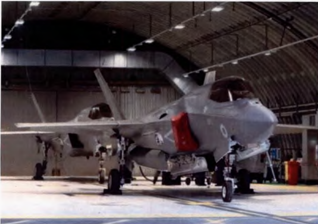
Figure 1.3.7 – Wrap around intake cover fitted to 617 Sqn aircraft at RAF Marham.
