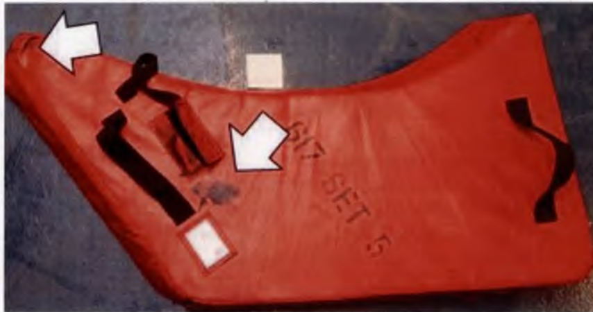
Figure 1.4.22 – BK-18 left intake blank. Arrows show black marks which were subject to chemical analysis.
