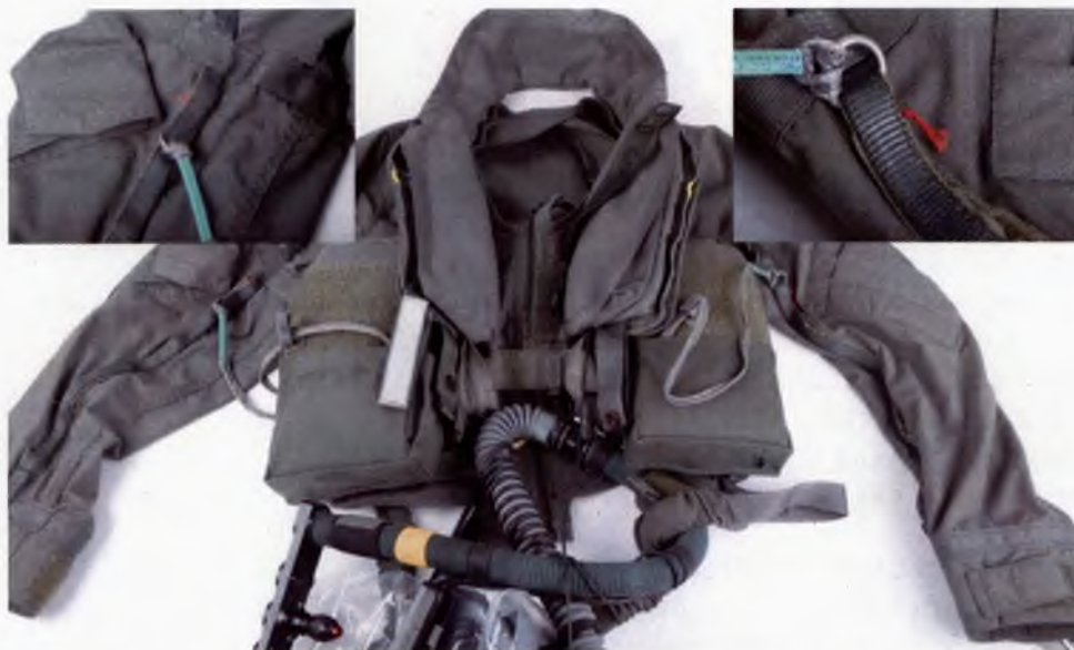
Figure 1.4.6 – BK-18 pilot’s flight jacket. AREL red tie on left sleeve remained intact.
