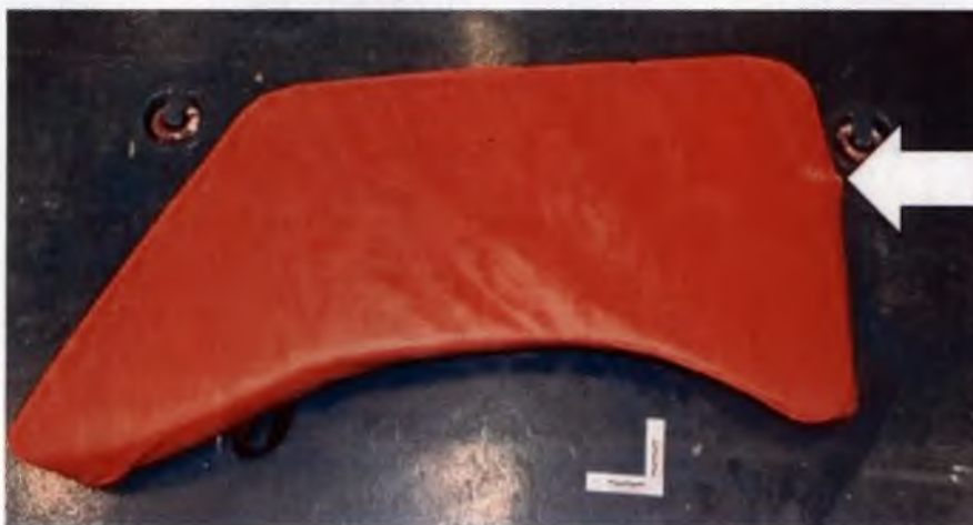
Figure 1.4.23 – Cuts to the top edge of BK-18 left intake blank.
