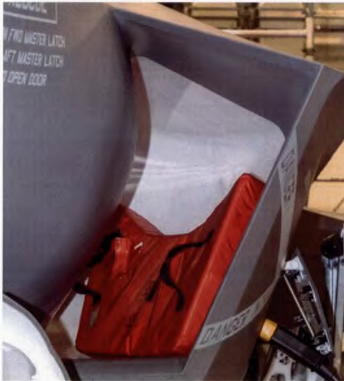
Figure 1.4.30 – Intake blank orientation after displacement.
