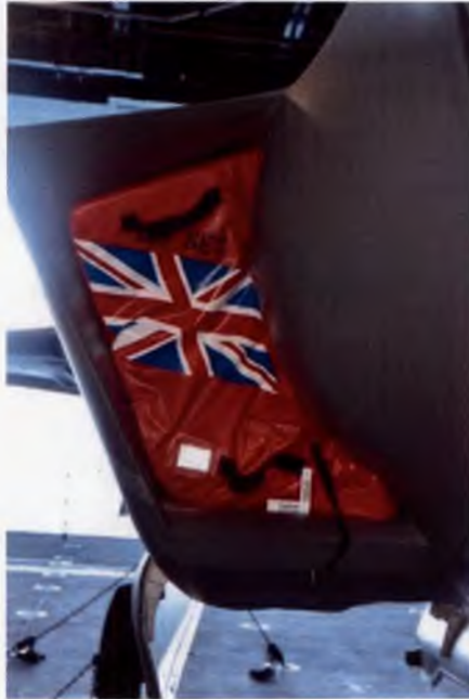
Figure 1.3.9 – Plug-type intake blank of the approved design, as used on Op FORTIS.
