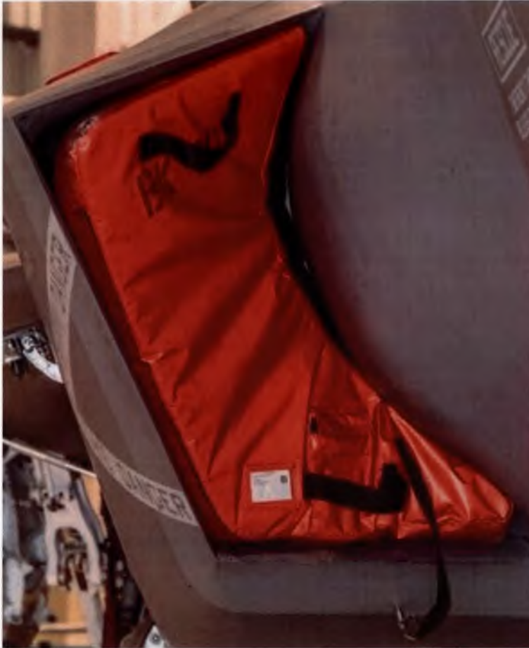
Figure 1.4.26 – Example of poorly installed intake blank seen at RAF Marham.
