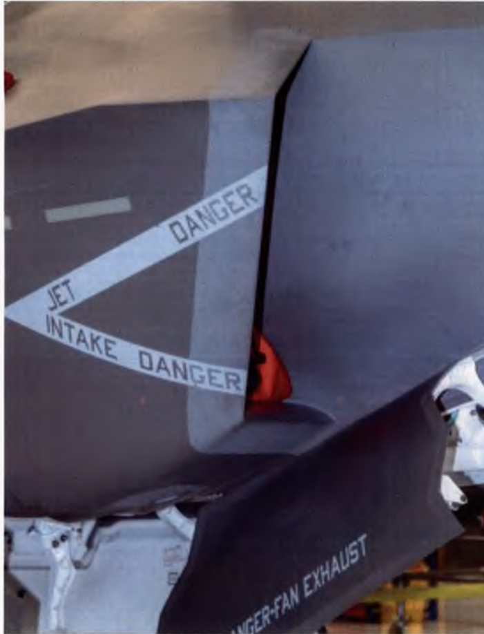
Figure 1.4.27 – Blank fitted using Lockheed Martin engineering test plan. Intake blank inboard lower edge remains exposed.
