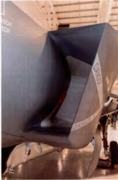
Figure 1.4.8 – Intake blank positioned in the intake.
