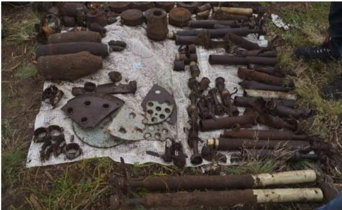
Figure 22: Other finds of explosive remnants of war, here artillery shells, missiles, fuzes, etc. For further explanations, see text.
