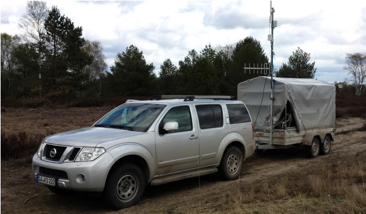
Figure 10: Workplace of the operator of the remote-controlled caterpillar with wireless antennas, generator (on trailer). For further explanations, see text.
