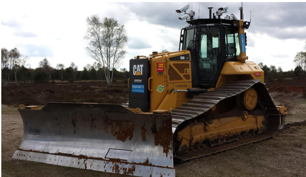
Figure 9: Unmanned, remote-controlled caterpillar used to create the fire-breaks surrounding the area suspected to be contaminated with cluster munitions. For further explanations, see text.
