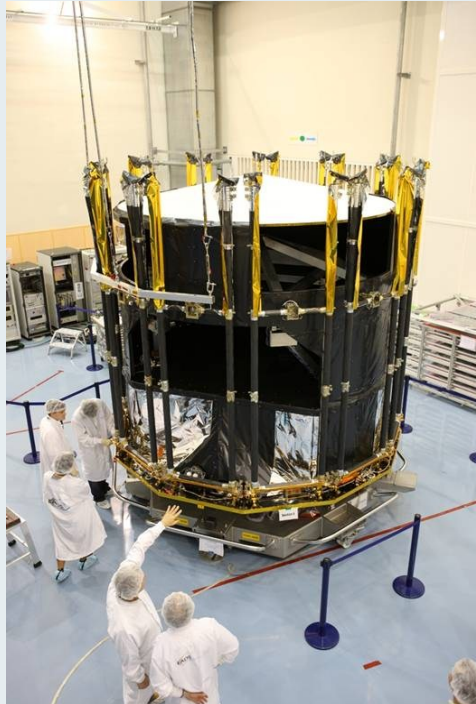
Gaia spacecraft equipped with a PLM mechanical dummy is being prepared for the mechanical test campaign (October 2011)
