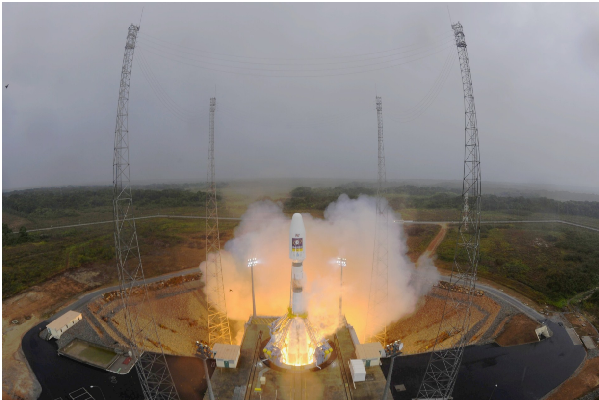
Soyuz boosters and main stage ignition seconds before liftoff on 21 October 2011. Boosters burn for about 2 mn before being jettisoned. Similar scenario should happen with Gaia in less than two years (Photo: ESA - S. Corvaja, 2011).
