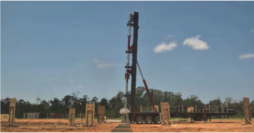
Figure 2. Kinetic impact test conducted in partnership with the U.S. Army Engineer Research and Development Center's Mobile Ballistic Research System at Fort Polk, Louisiana
