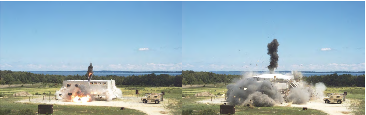
Figure 4. Two-story over-burial building debris test at Aberdeen Proving Ground, Maryland
