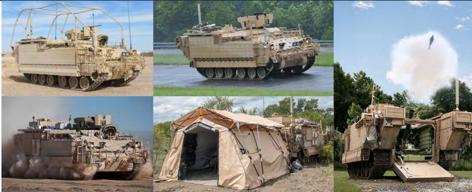
Armored Multi-Purpose Vehicle uses, clockwise from top left: General Purpose | Mission Command | Mortar Carrier | Medical Treatment with Shelter | Medical Evacuation
