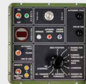
Loading unit control panel
