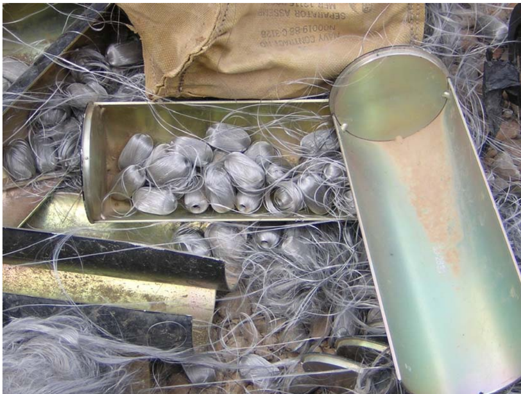
The United States dropped these carbon fiber filaments in an attack on electrical power in al-Nasiriyya. These filaments are designed to disable power, but in this case they caused a fire that destroyed the transformer station and plunged the city into darkness for thirty days. © 2003 Marc Garlasco / Human Rights Watch
