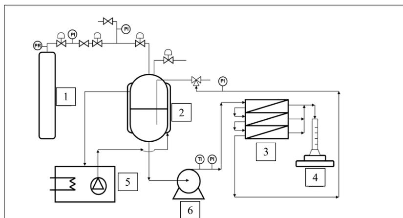
**Figure 1.** Flow diagram of the Triple System Model F1 membrane module designed by Hidalgo et al. [19]: (1) nitrogen bottle (outer cage); (2) feed tank; (3) membrane Triple System Model F1; (4) digital scale; (5) thermostat; (6) pressure pump.
