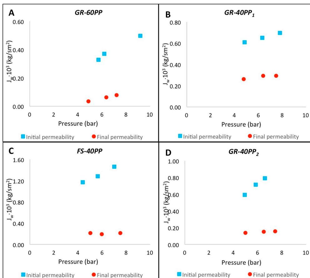
**Figure 4.** Comparison of water mass fluxes before and after clarification of pomegranate juice for GR-60PP (A), GR-40PP<sub>1</sub> (B), FS-40PP (C) and GR-40PP<sub>2</sub> (D) membranes.
