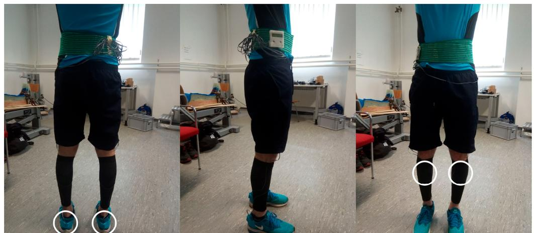
**Figure 1.** Full IMU setup. White circles indicate the positions of the placed sensors used for analysis.
