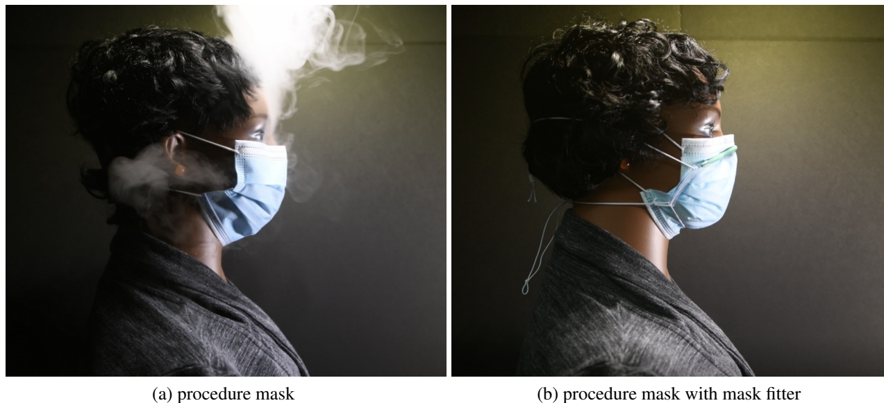
Figure 8: Visualization illustrating aerosol leakage for the procedure mask (a) mask as typically worn (b) mask with Badger Seal mask fitter installed.
