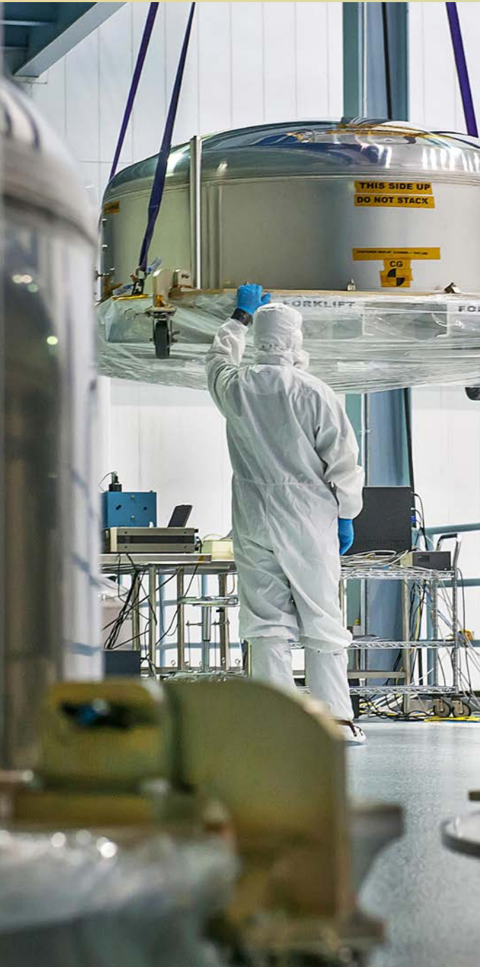
An engineer guides one of the canisters containing a mirror segment for NASA's James Webb Space Telescope. (NASA/Desiree Stover)
