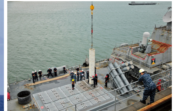
The photo on the left shows a SM-2 missile being fired from the VLS of Arleigh Burke-class missile destroyer USS Benford. The VLS (Vertical Launching System) is the section that looks like a grid on the ship deck seen below. Each grid is called a "cell," inside which is a canister containing a missile stored vertically. The VLS of Japan's most advanced Maya-class Aegis ship carries a total of 96 cells on the front and rear decks. If the ship carries only surface-to-air missiles (SAMs), this means 96 SAMs could be fired to intercept - but usually other missiles such as anti-submarine missiles are installed in a certain number of cells. (Photo Credit: U.S. Navy)
