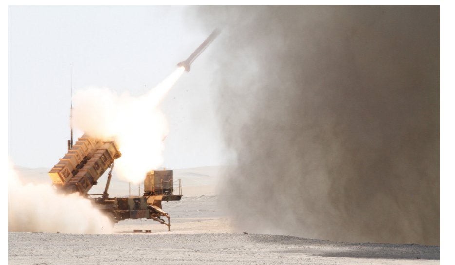
A Patriot missile launcher fires a PAC-2 missile. One launcher carries four canisters. One canister can carry one PAC-2 missile or four PAC-3 missiles. Therefore, one launcher can carry four PAC-2 missiles or 16 PAC-3 missiles at a maximum. (Photo Credit: U.S. Army)
