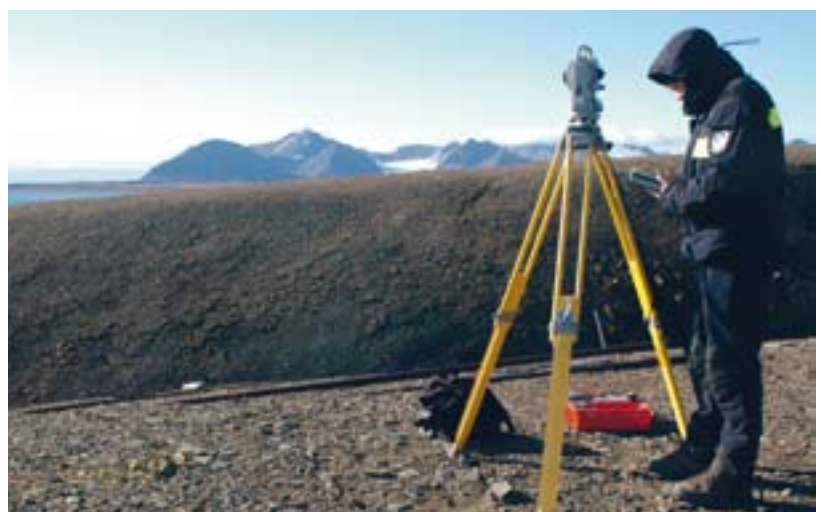
Figure 5 Wouter Ytsma, University of Groningen, mapping a mining camp with total station – a highly accurate instrument used for mapping archaeological sites. Photo: Dag Avango.
