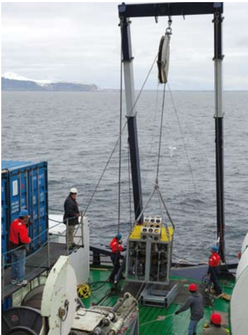
Figure 5 The CAMPER wireline vehicle being lowered over the side during a test dive off Bear Island. Photo: Björn Eriksson.
