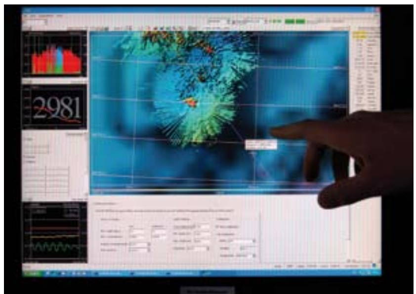
Figure 4 Photo showing the data acquisition window of Oden’s EM120 multibeam system. The example shows how bathymetric data was collected in a 360° sector around the ship, referred to as “pirouette surveying” (see text for explanation). This way of carrying out multibeam mapping worked well in hard ice conditions where the heavy ice breaking otherwise significantly disturbed the data acquisition. Photo: Martin Jakobsson.
