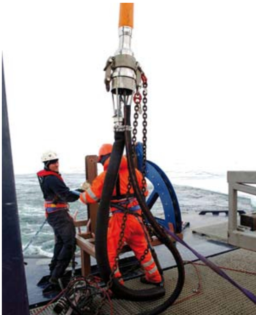
Figure 2 Launching of the seismic equipment: Airgun cluster lower left and umbilical head above the two participants. Photo: Trine Dahl-Jensen.
