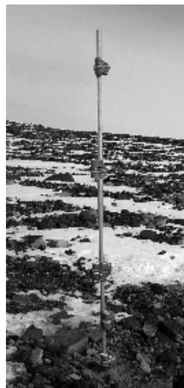
Figure 3 Installed dataloggers for short term monitoring of climate parameters in relation to frost heave landforms at Wasa. Photo: Hanna Ridefelt.
