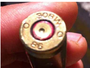
Photo 26 Czechoslovakian .308 Winchester cartridge case produced in 1986 by Sellier & Bellot.
