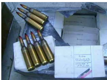
Photo 34 Iraqi 14.5×114mm armour-piercing incendiary (API) cartridges produced by the Al Yarmouk State Establishment.
