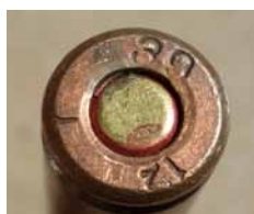
Photo 10 Sudanese 7.62×39 mm cartridge produced in 2012 by the Military Industry Corporation.
