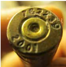
Photo 3 Iranian 7.62×39 mm cartridge case produced in 2001 by the Defense Industries Organization's Ammunition & Metallurgy Industries Group.
