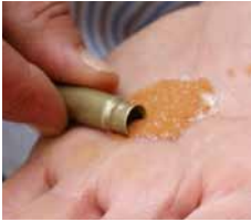
Photo 20 Booby-trapped ammunition observed in Deir Sonbul. Note the granular white and rust-coloured substances in place of propellant.
