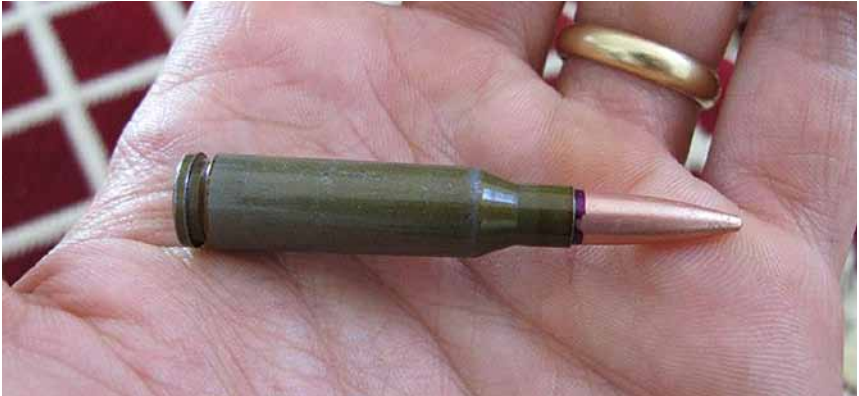
Photo 41 Russian 5.45×39 mm FMJ cartridge produced in 1998 by Barnaul Machine Tool Plant JSC. © Damien Spleeters
