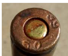
Photo 11 Sudanese 7.62×39 mm cartridge produced in 2009 by the Military Industry Corporation. Note the lack of a third entry in the headstamp.
