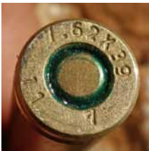
Photo 4 Iranian 7.62×39 mm cartridge produced in 2011 by the Defense Industries Organization's Ammunition & Metallurgy Industries Group. Note three-entry type headstamp.
