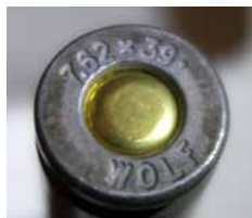
Photo 12 WOLF brand 7.62 × 39 cartridge likely manufactured at either Ulyanovsk Machinery Plant or Tula Cartridge Works, both located in the Russian Federation, prior to 2009.
