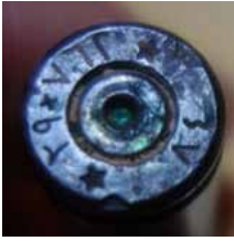
Photo 1 Syrian 7.62×39 mm cartridge case produced in 1984 by the Industrial Establishment of Defense (EID) in Damascus, showing earlier-style production characteristics.
