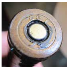
Photo 31/32 Chinese 14.5 × 114 mm BZT armour-piercing incendiary tracer (API-T) cartridge produced in 1972 by State Factory 631.
