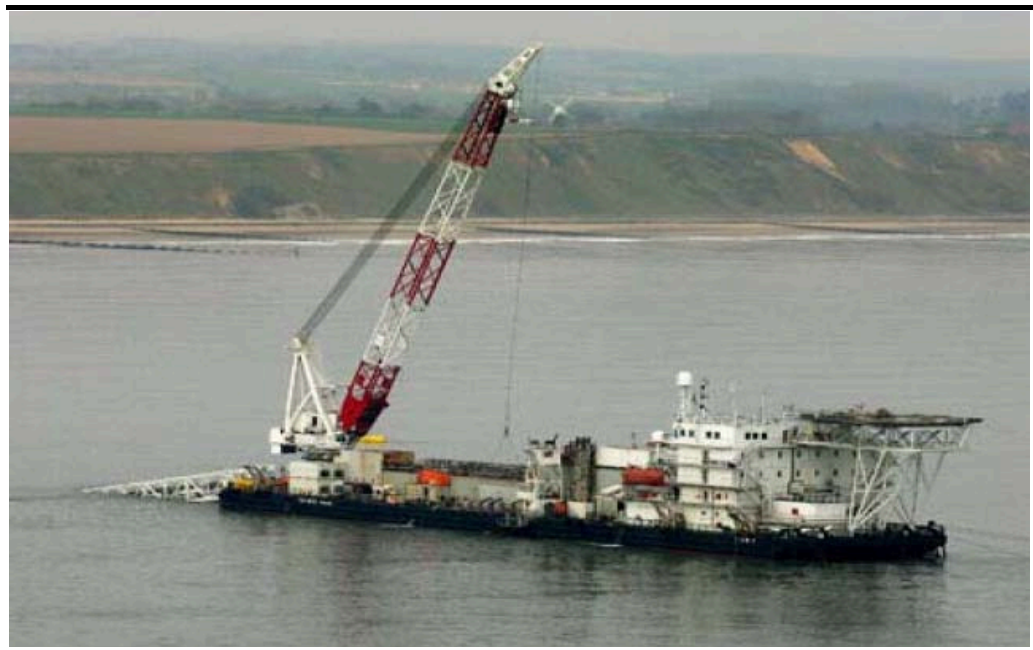
Figure 4.5 Standard Shallow Water Pipe Lay Barge
