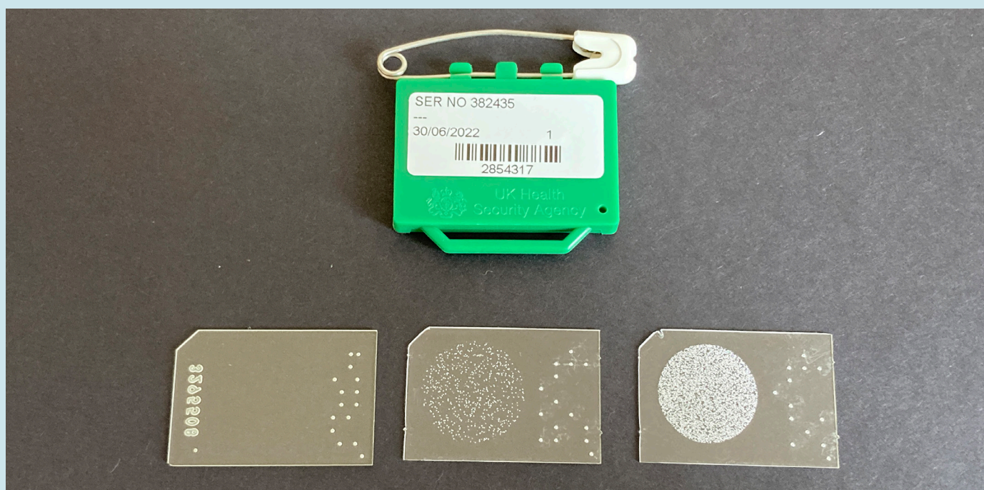
PADC dosimeter top, PADC plastic below, before and after processing
