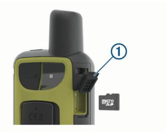
2 Insert the memory card with the gold contacts facing the front of the device.
