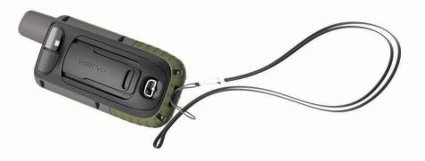
2 Thread the other end of the strap through the loop, and pull it tight.
