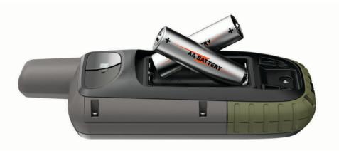
3 Replace the battery cover, and turn the D-ring clockwise.
